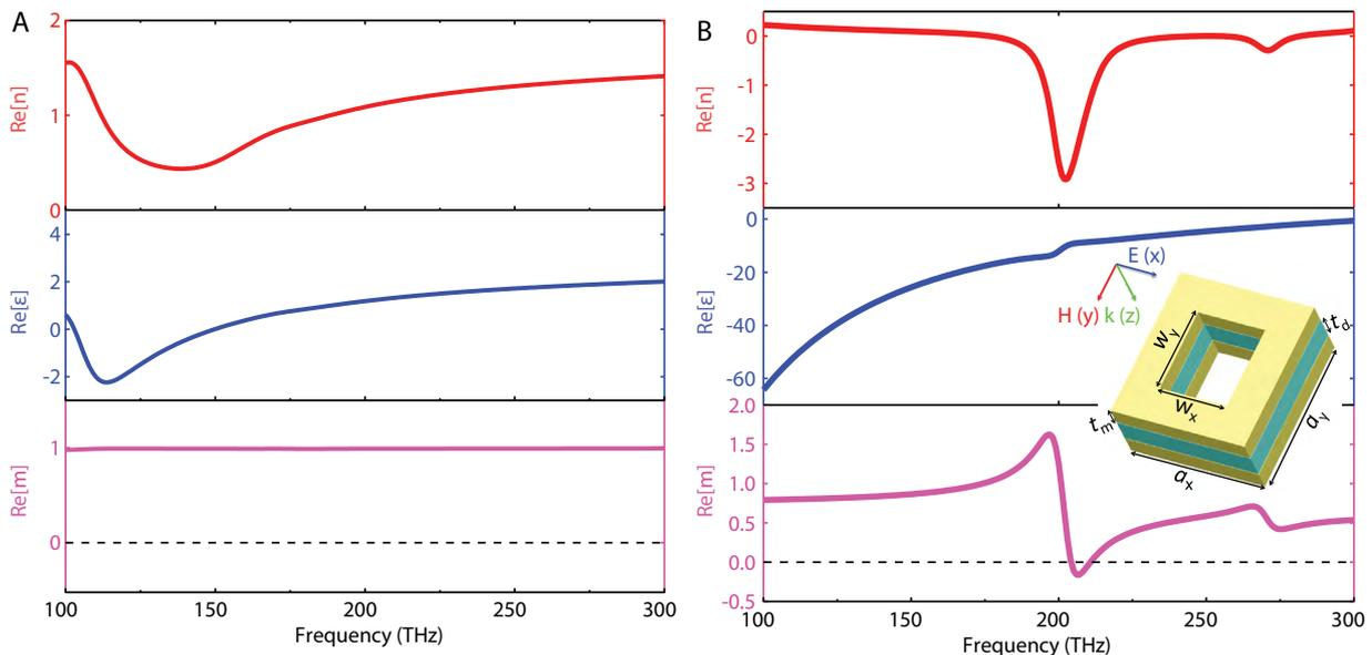
**Figure 2** Retrieved real part of effective refractive index  $[\text{Re}(n)]$ , permittivity  $[\text{Re}(\epsilon)]$ , and permeability  $[\text{Re}(\mu)]$  for fishnet structure made by AZO-MgO-AZO (A) and Au-MgO-Au (B), respectively. The fishnet structure [schematically shown as inset of Figure 2(B)] has dimensions  $a_x=500$  nm,  $a_y=600$  nm,  $w_x=200$  nm,  $w_y=350$  nm,  $t_m=30$  nm, and  $t_d=40$  nm.
