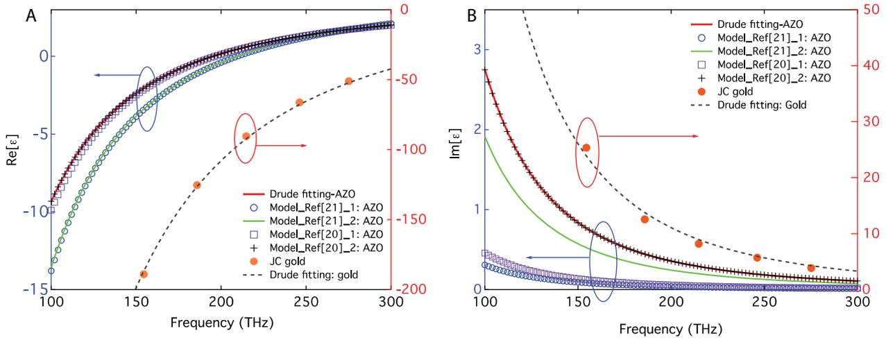
**Figure 1** Comparison of data for gold and AZO between 100 and 300 THz: (A)  $\text{Re}(\epsilon)$  and (B)  $\text{Im}(\epsilon)$ . For AZO, our fitted Drude model is listed together with the models in Refs. [21] and [24] w/ and w/o a  $2\pi$  factor taken into account in the corresponding collision frequency. For gold, our Drude fitted model is shown consistent with experimental data by Johnson and Christy [22].
