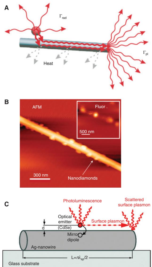
**Figure 3:** Experimental approaches on random single emitter surface plasmon coupling. (A) Single CdSe colloidal QDs are placed next to single silver nanowires, separated by a PMMA spacer layer from the nanowire [45]. (B) AFM image of a silver nanowire with adhered nanodiamonds containing single NV centers [41]. (C) CdSe colloidal QDs placed on a silver nanowire, separated by a  $\text{SiO}_2$  spacer layer [46].
