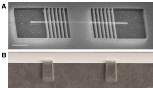
**Figure 7:** Plasmon resonators made (A) on a silver colloidal nanowire by defining DBR mirrors on the surrounding PMMA medium [61] and (B) by adding block reflectors confining a plasmon mode propagating along the wedge [64]. The scale bars in (A) and (B) both correspond to 1  $\mu\text{m}$ .
