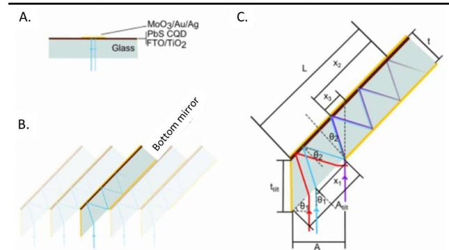
**Fig. 7.** Configuration and geometric considerations in FLP CQD solar cells. (A) Conventional double-pass CQD solar cell configuration. (B) Periodic arrangement of FLP CQD solar cells. (C) Geometric considerations for multipass absorption in the FLP cell. Reprinted with permission from [236]. Copyright 2013 Macmillan Publishers Ltd.
