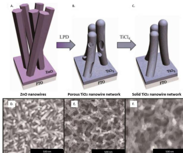
**Fig. 3.** Fabrication procedure for  $\text{TiO}_2$  nanowire network electrodes for CQD BH solar cells. (A, D) ZnO nanowires were first synthesized on an FTO substrate via a hydrothermal method. (B, E) The ZnO nanowires were converted to porous  $\text{TiO}_2$  nanowire networks via LPD. (C, F) Solid  $\text{TiO}_2$  nanowire networks were formed as a result of  $\text{TiCl}_4$  treatment. Reprinted with permission from [209]. Copyright 2013 Wiley-VCH Verlag GmbH & Co. KGaA.
