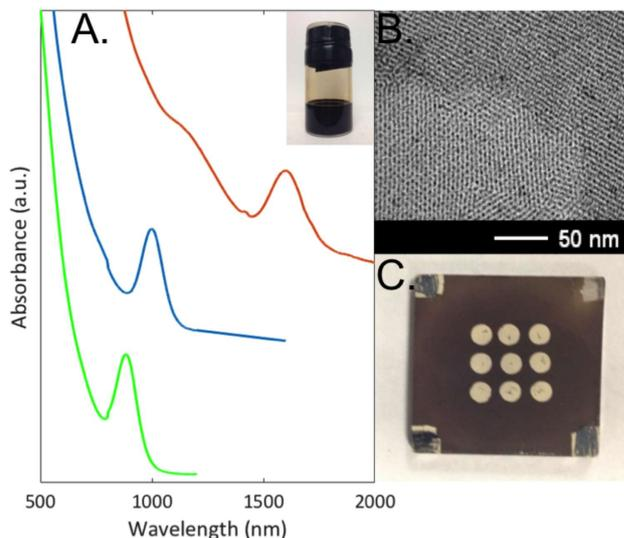
**Fig. 1.** (A) Solution-phase absorption spectra of PbS CQDs with excitonic peaks at wavelengths of 880, 1000 and 1600 nm. Spectra are offset for clarity. Inset: photograph of as-synthesized PbS CQD solution with excitonic peak at 955 nm. (B) Transmission electron microscope image of a large ensemble of PbS CQDs with excitonic peak wavelength of 950 nm. (C) Top-view photograph of a  $3 \times 3$  array of PbS CQD photovoltaic cells (full substrate is 1 inch  $\times$  1 inch).
