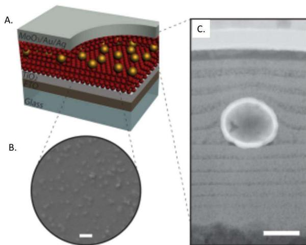
**Fig. 8.** Plasmonic–excitonic solar cell device design. (A) Schematic of the PbS CQD DH device with embedded nanoshells. (B) Top view scanning electron microscope image showing representative density of nanoshells after CQD deposition. Scale bar, 1  $\mu\text{m}$ . (c) Cross-sectional TEM image showing a single gold nanoshell embedded in a PbS CQD film. Scale bar, 100 nm. Reprinted with permission from [240] Copyright 2013 American Chemical Society.
