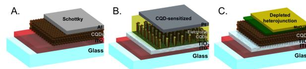
**Fig. 2.** Schematics of different CQD solar cell architectures employing: (A) a Schottky junction, (B) CQDs as sensitizers, (C) a depleted heterojunction.
