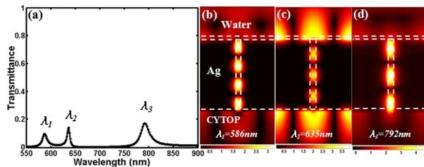
**Fig. 2.** Transmission spectrum of nanoslit arrays with  $P = 500$  nm,  $D = 460$  nm,  $W = 25$  nm,  $t = 20$  nm (a). Calculated magnetic field distributions at resonant peaks of  $\lambda_1$  (b), and  $\lambda_2$  (c),  $\lambda_3$  (d), respectively. The white dotted lines mark the boundaries of the structure.
