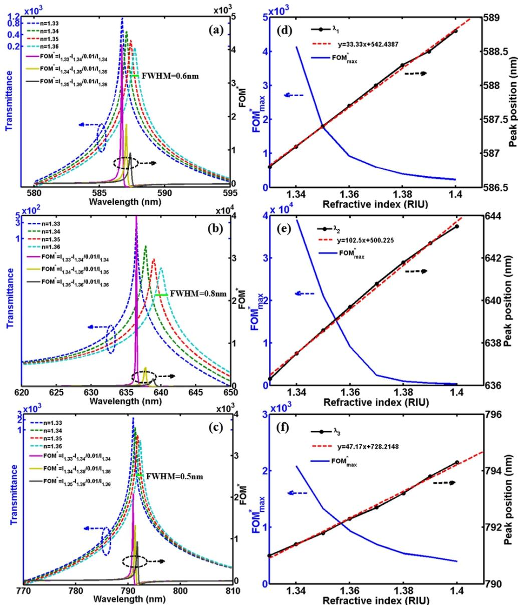
**Fig. 7.** (a)–(c) Transmission spectra and FOM\* of the resonant peaks ( $\lambda_1 - \lambda_3$ ) when the structure is immersed in sodium chloride–water mixture solutions with varying concentrations. (d)–(f) The FOM\*<sub>max</sub> and peak positions for the resonant peaks ( $\lambda_1 - \lambda_3$ ) as a function of the varying RI, respectively.
