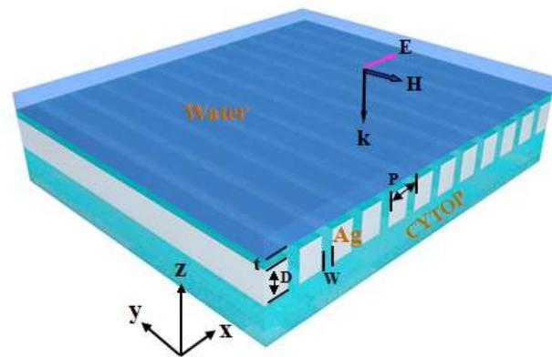
**Fig. 1.** Schematic of a metallic nanoslit arrays embedded in the CYTOP, with the geometrical parameters ( $t$ ,  $D$ ,  $W$  and  $P$ ), and the direction of the TM-polarized incident light.
