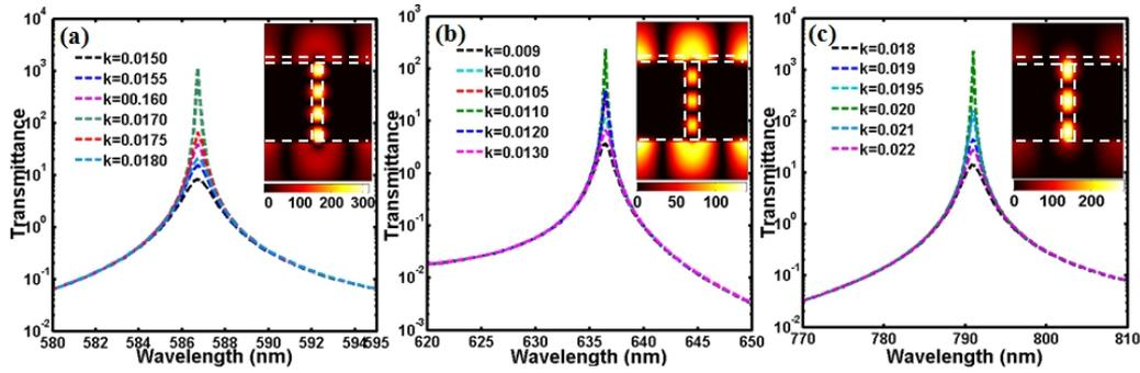
**Fig. 6.** Transmittance spectra of different gain values assisted nanoslit array for  $\lambda_1 - \lambda_3$ , respectively. The inset in (a)–(c) show the enhanced magnetic field distributions of the structure at corresponding gain threshold for  $\lambda_1 - \lambda_3$ .
