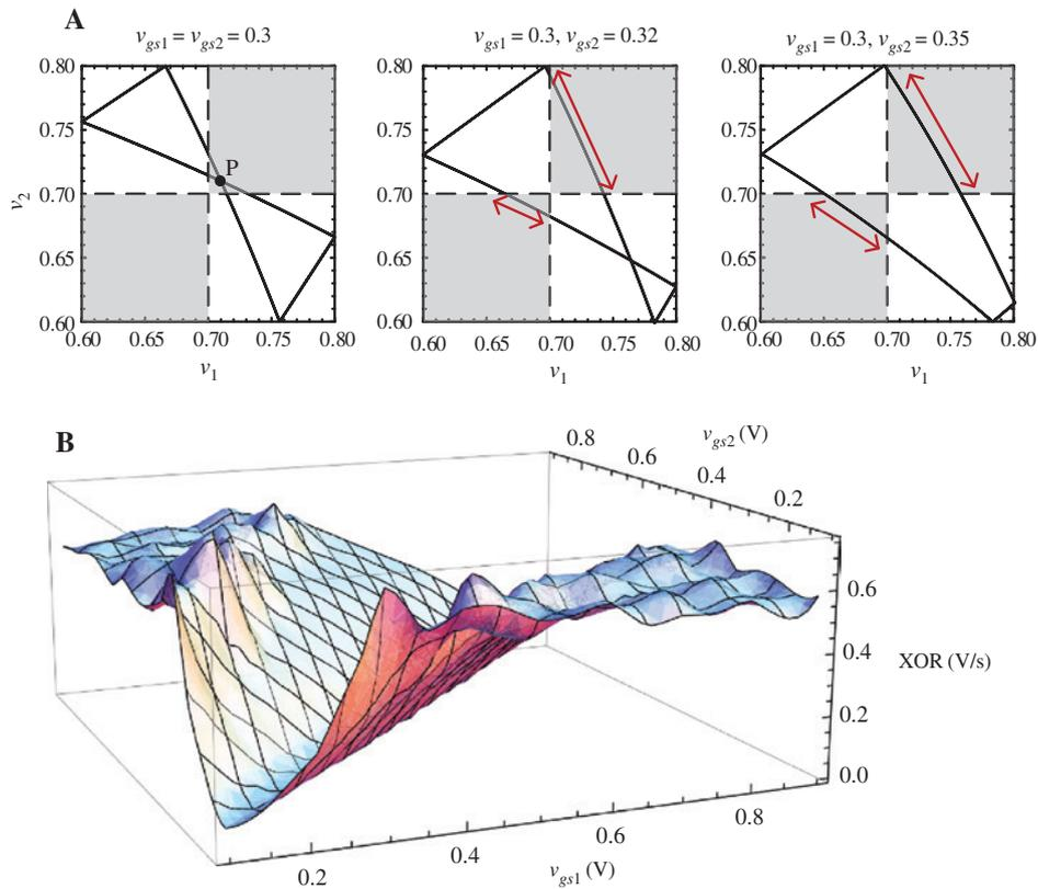
**Figure 4:** (A) Relationship between XOR output and the steady-state periodic orbit of the system. At any instant of time, XOR output is 1 in the grey region and 0 otherwise. Averaged XOR output is equal to the fraction of time spent by the system in the grey regions. XOR output is minimum in case of a butterfly-shaped orbit (left) and should increase as the orbit transitions to a rectangular orbit (right). (B) XOR surface as a function of  $v_{gs1}$  and  $v_{gs2}$ .
