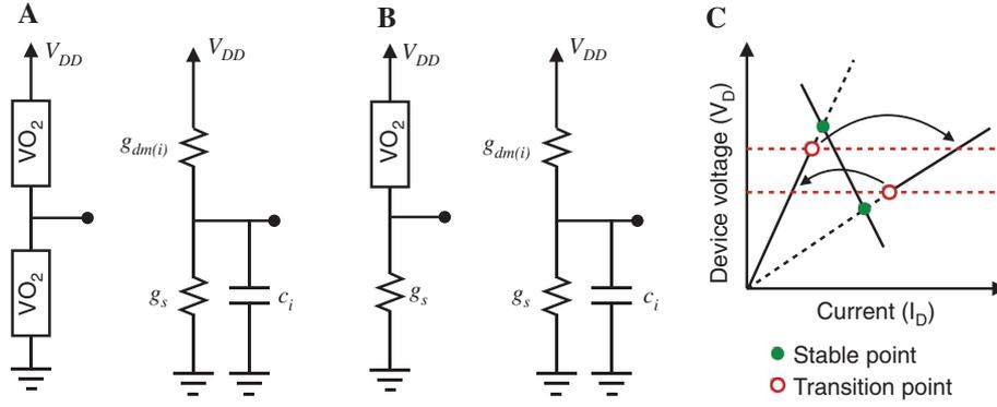
**Figure 1:** (A) D-D oscillator circuit configuration and its equivalent circuit. (B) D-R oscillator circuit configuration and its equivalent circuit. (C) Load line graph for the D-R circuit and the region of operation of D-R oscillator. When the stable points (green filled points) are outside the region of operation, the system shows oscillations.
