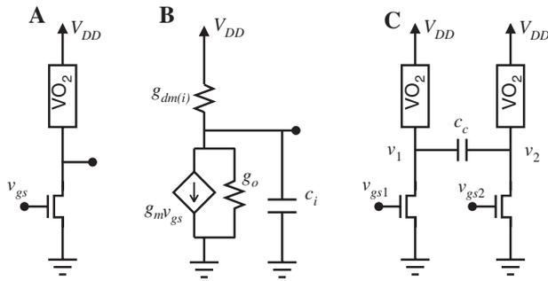
**Figure 3:** (A) Oscillator circuit with MOSFET in series with a  $VO_2$  device. (B) Small signal equivalent circuit of the oscillator with  $VO_2$  in series with a MOSFET. (C) Coupled oscillator circuit with a series MOSFET in place of a series resistance.
