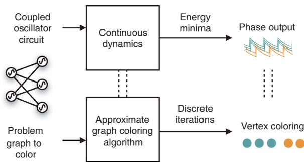
**Figure 7:** Overview of the proposed graph coloring system using coupled  $\text{VO}_2$  oscillators where each node corresponds to a  $\text{VO}_2$  oscillator. The dynamics of the system corresponds to an approximate graph coloring algorithm, and as such, the steady-state phase output of the  $\text{VO}_2$  oscillators can be used to color the nodes of the graph.
