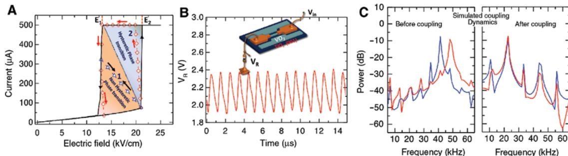
**Figure 5:** (A) Measured I-E characteristics of a  $\text{VO}_2$  device illustrating the hysteretic window. (B) Measured characteristics show oscillations when biased with a pull-down resistor. (C) Measurements and simulations illustrate frequency locking when two oscillators are coupled electrically.
