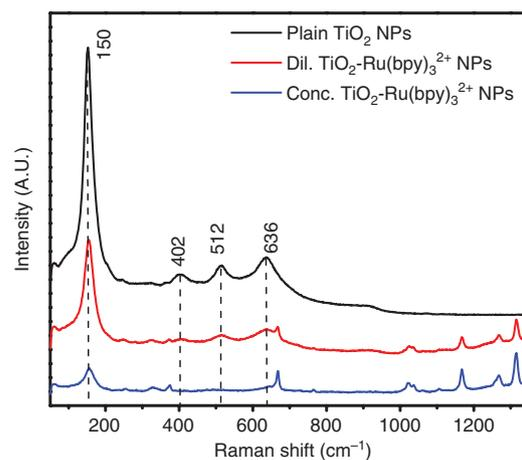
**Figure 5:** Raman spectra of the plain  $\text{TiO}_2$ , diluted  $\text{TiO}_2\text{-Ru}(\text{bpy})_3^{2+}$  and concentrated  $\text{TiO}_2\text{-Ru}(\text{bpy})_3^{2+}$  NPs.
