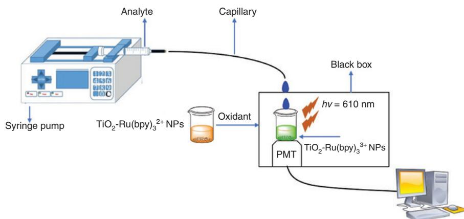
**Figure 1:** A schematic representation of the experimental setup and reaction scheme for the  $\text{TiO}_2\text{-Ru}(\text{bpy})_3^{2+}$  solid-state CL sensor.
