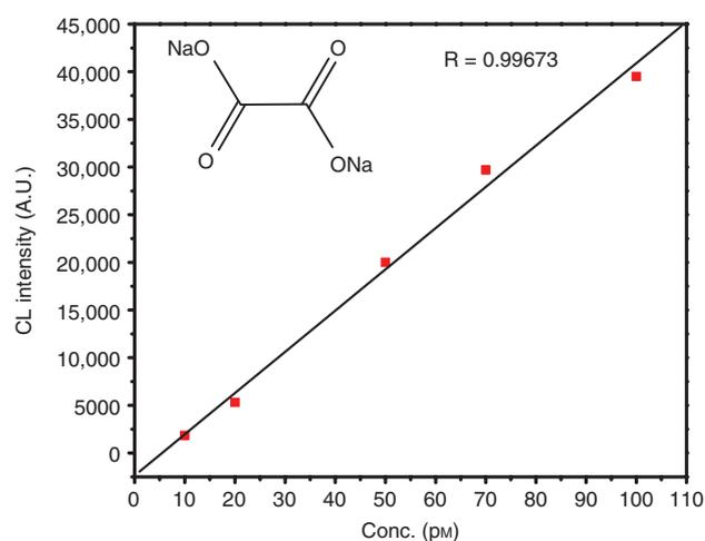
**Figure 9:** Calibration curve obtained for sodium oxalate using diluted  $\text{TiO}_2\text{-Ru}(\text{bpy})_3^{2+}$  NPs. Conditions: 0.5 mM Ce(IV) and 200 ml/h flow rate. The oxalate structure is also shown.
