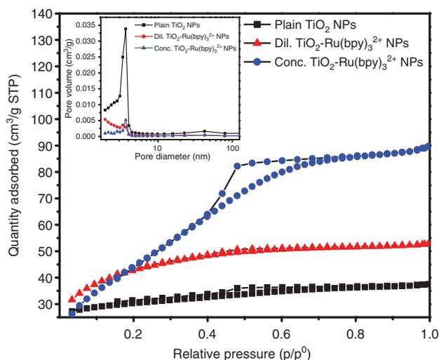
**Figure 3:** N<sub>2</sub> adsorption-desorption isotherms of the plain TiO<sub>2</sub>, diluted and concentrated TiO<sub>2</sub>-Ru(bpy)<sub>3</sub><sup>2+</sup> NPs. The inset is the pore size distributions for the samples.
