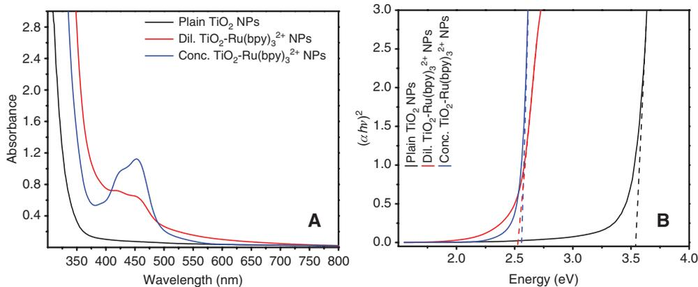
**Figure 4:** (A) UV-Vis absorption spectra of the plain  $\text{TiO}_2$ , diluted  $\text{TiO}_2\text{-Ru}(\text{bpy})_3^{2+}$  and concentrated  $\text{TiO}_2\text{-Ru}(\text{bpy})_3^{2+}$  NPs. (B) A plot of  $(\alpha h\nu)^2$  vs.  $h\nu$  for the plain  $\text{TiO}_2$ , diluted  $\text{TiO}_2\text{-Ru}(\text{bpy})_3^{2+}$  and concentrated  $\text{TiO}_2\text{-Ru}(\text{bpy})_3^{2+}$  NPs.
