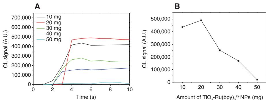
**Figure 8:** (A) The individual CL signal vs. time using different amounts of  $\text{TiO}_2\text{-Ru}(\text{bpy})_3^{2+}$  NPs. (B) The effect of the amount of  $\text{TiO}_2\text{-Ru}(\text{bpy})_3^{2+}$  NPs (mg) using oxalate as an analyte at a flow rate of 200 ml/h.
