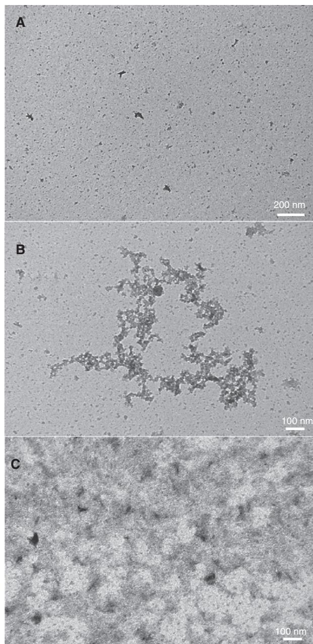
**Figure 2:** TEM images of the (A) plain TiO<sub>2</sub> and (B) diluted and (C) concentrated TiO<sub>2</sub>-Ru(bpy)<sub>3</sub><sup>2+</sup> NPs.
