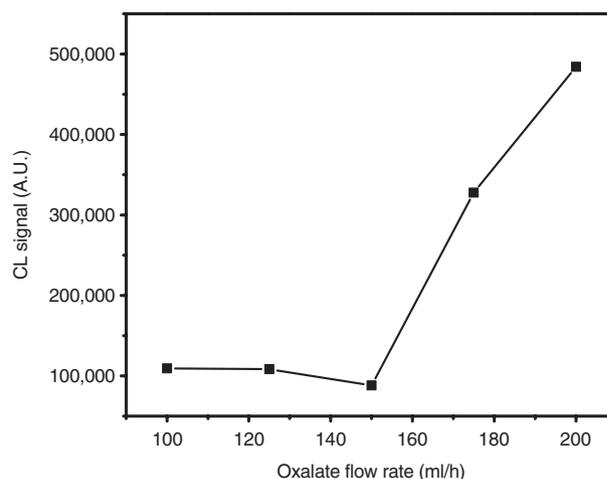
**Figure 7:** The effect of analyte (oxalate) flow rate (ml/h) on CL signal using diluted TiO<sub>2</sub>-Ru(bpy)<sub>3</sub><sup>2+</sup> NPs.
