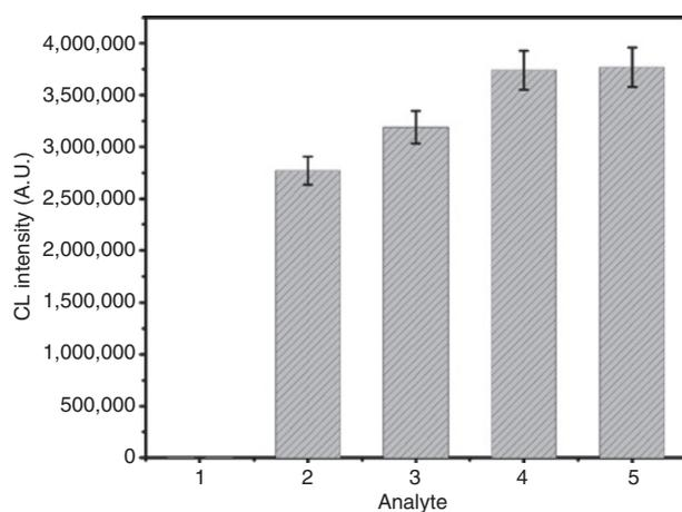
**Figure 6:** The CL signal detected using 0.5 mM Ce(IV) in 0.25 M sulfuric acid as oxidant and 1 mM oxalate as the analyte: 1, plain TiO<sub>2</sub> NPs; 2, concentrated Ru(bpy)<sub>3</sub><sup>2+</sup> aqueous solution; 3, diluted Ru(bpy)<sub>3</sub><sup>2+</sup> aqueous solution; 4, concentrated TiO<sub>2</sub>-Ru(bpy)<sub>3</sub><sup>2+</sup> NPs; 5, diluted TiO<sub>2</sub>-Ru(bpy)<sub>3</sub><sup>2+</sup> NPs.
