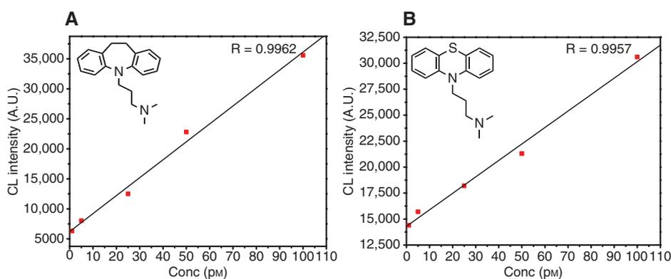
**Figure 10:** Calibration curve for (A) imipramine drug and (B) promazine drug. Conditions: 0.5 mM Ce(IV) and 200 ml/h flow rate. The structures of the drugs are also shown.
