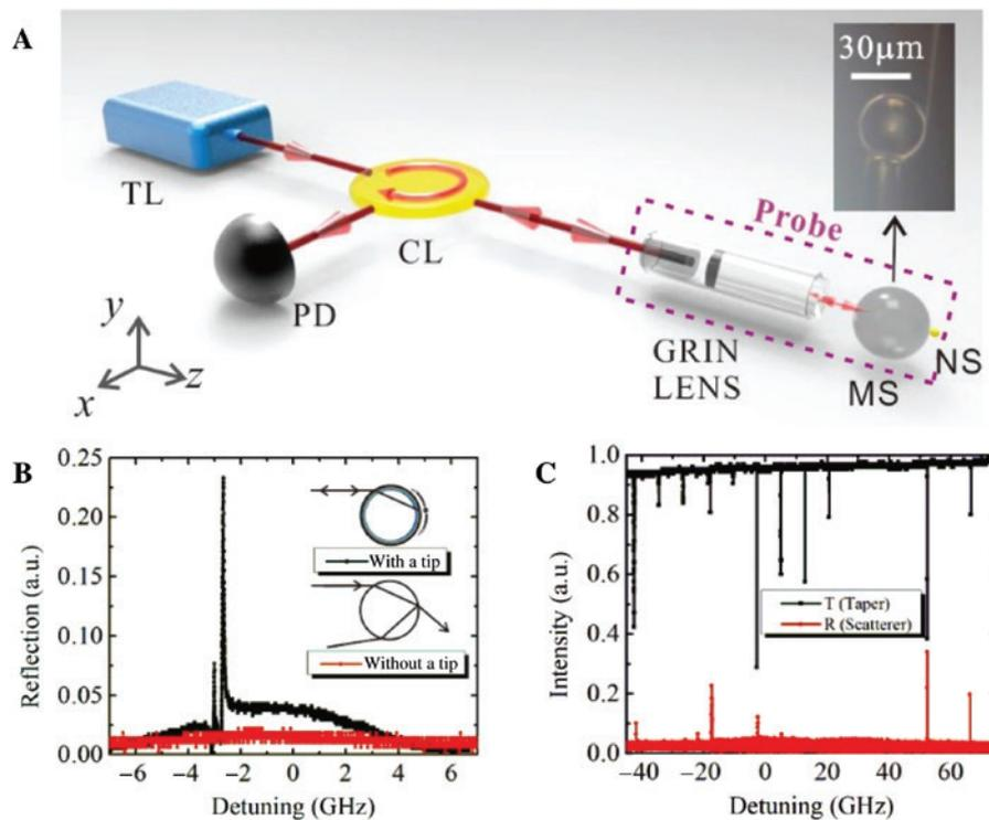
**Figure 1:** (A) Illustration of the experimental setup.
