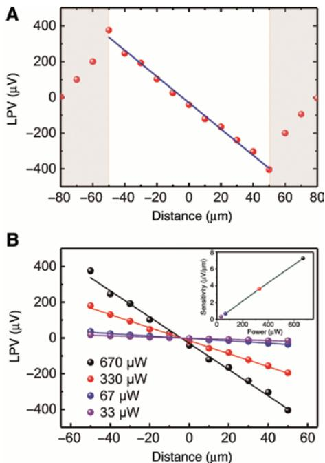
**Figure 4:** Lateral photovoltaic effect for the laser-scribed rGO devices: (A) LPV at different positions of laser spots (633 nm) and (B) LPV between the two Au electrodes with different laser powers. The inset is the sensitivity at different laser powers.
