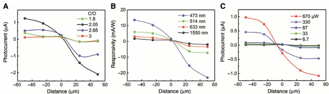
**Figure 3:** Photoresponse of rGO films at different positions of laser spots with (A) different C/O ratios (473 nm laser), (B) different laser wavelengths, and (C) different laser powers at 633 nm.
