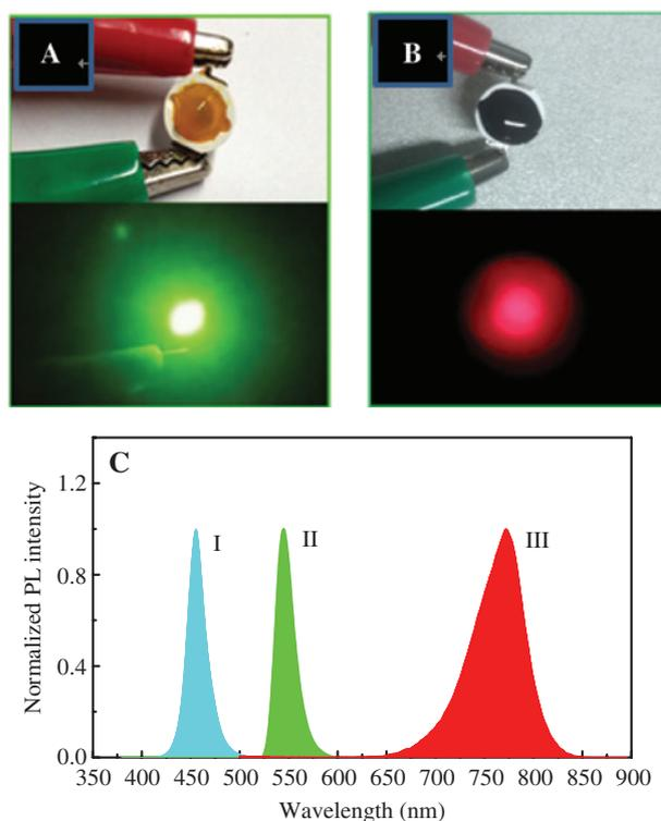
**Figure 6:** Photographs of (A) the MAPbBr<sub>3</sub>/PDMS-urea gel and (B) the MAPbI<sub>3</sub>/PDMS-urea gel-coated GaN LEDs under the operation potential of 2.7 V and (C) Emission spectra of the blue GaN LED (I), the MAPbBr<sub>3</sub>/PDMS-urea gel coated green LED (II) and the MAPbI<sub>3</sub>/PDMS-urea gel coated red LED (III).
