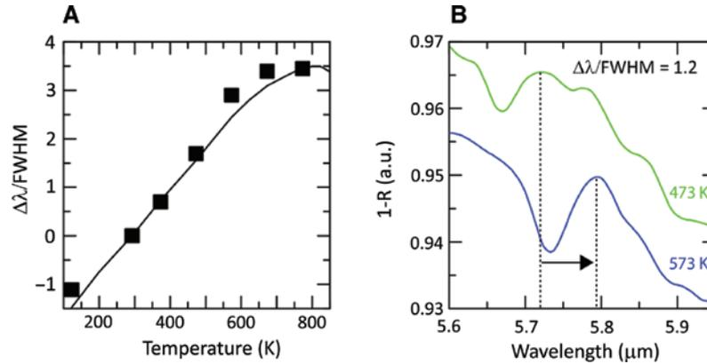
**Figure 3:** Normalized tunability ( $\Delta\lambda/\text{FWHM}$ ) of high-order MO mode in the Ge resonator. (A) Temperature-dependent MO shifts normalized to the resonance linewidth. (B) Tuning by more than one resonance linewidth ( $\Delta\lambda/\text{FWHM} = 1.2$ ) with a  $\Delta T = 100$  K temperature gradient.
