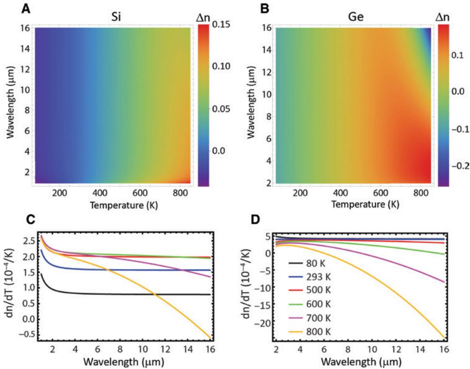
**Figure 1:** Temperature and wavelength dispersion of  $n$  and  $dn/dT$  in Silicon and Germanium. Thermally induced index shifts in Si (A) and Ge (B) as a function of wavelength (2–16  $\mu\text{m}$ ) and temperature (80–850 K). (C) and (D) The chromatic dispersion of  $dn/dT$  at various temperatures in Si (C) and Ge (D). Each color plot corresponds to  $dn/dT$  at different temperatures as detailed in the legend of (D).
