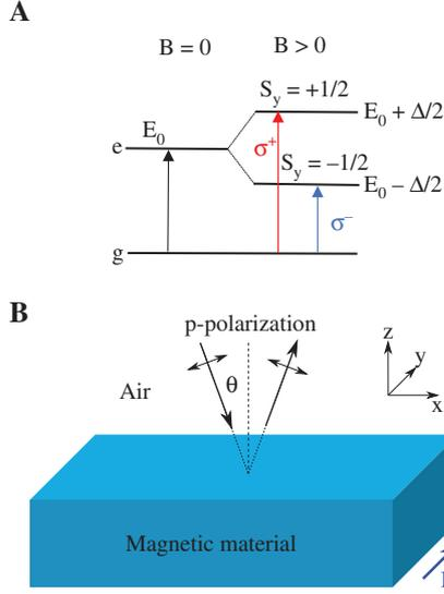
**Figure 1:** (A) Scheme of the optical transitions in a three-level system composed of the ground level (g) and two excited states (e), which are split off due to the Zeeman effect in magnetic field  $B \parallel y$ . (B) Geometry of the considered setting, where  $p$ -polarized light is reflected from a semi-infinite magnetic medium with a three-level resonance shown in (A).
