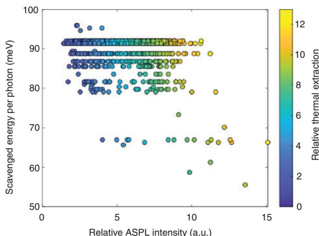
**Figure 3:** Relative ASPL intensity versus scavenged thermal energy per emitted photon for the sample with uniform Au nanoparticle coverage. The color of each point corresponds to the scavenged thermal energy per photon multiplied by the relative ASPL intensity and normalized to the average corresponding value for the control.
