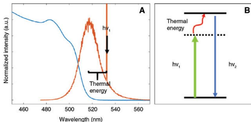
**Figure 1:** Illustration of anti-Stokes photoluminescence.
