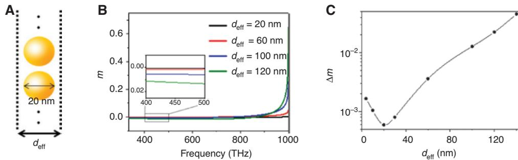
**Figure 2:** Error minimizing choices of the effective thickness  $d_{\text{eff}}$  and the branch  $m$ .
