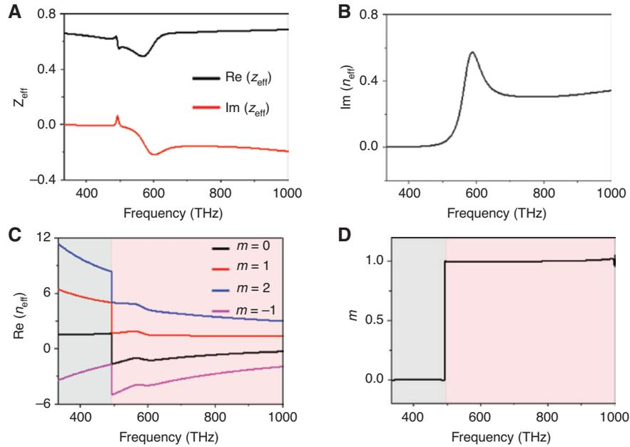
**Figure 4:** Effective parameters for the homogenized seven layers of gold nanoparticles.
