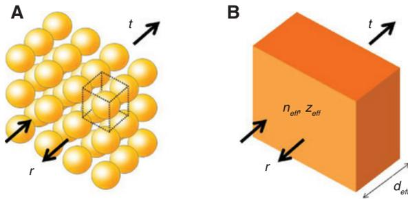
**Figure 1:** Homogenization of metamaterials. (A) Schematic of a gold nanoparticle array. (B) The homogenized slab with the effective parameters.  $r$  and  $t$  are the reflection and transmission coefficients, respectively.
