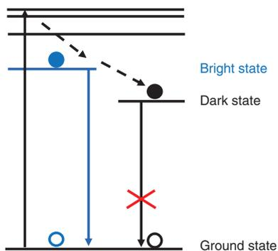
**Figure 3:** Possible dark exciton states in (iso-BA)<sub>2</sub>PbI<sub>4</sub> perovskite.
