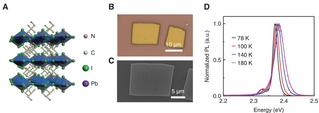
**Figure 1:** Crystal structure and PL spectra of (iso-BA)<sub>2</sub>PbI<sub>4</sub> perovskite crystals.
