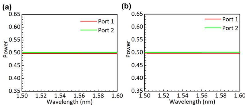
**Figure 6:** Simulated power splitting ratio of the designed power splitter for the  $TE_0$  (a) and  $TE_1$  (b) modes.
