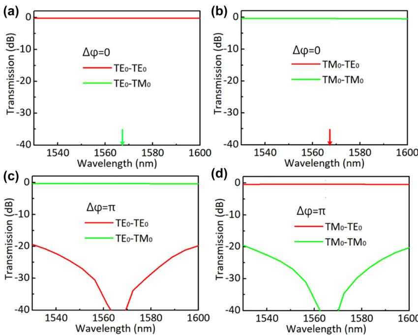
**Figure 8:** Simulated light transmissions of the designed polarization switch for the launched  $TE_0$  (a) and  $TM_0$  (b) modes with  $\Delta\phi = 0$ ; simulated light propagation of the designed polarization switch for the launched  $TE_0$  (c) and  $TM_0$  (d) modes with  $\Delta\phi = \pi$ .
