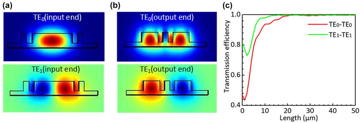
**Figure 4:** The mode profiles of the  $TE_0$  and  $TE_1$  modes at the input end (a) and the output end (b) of the triple-core waveguide of the PS. (c) Simulated conversion efficiencies of the  $TE_0-TE_0$  and  $TE_1-TE_1$  in the triple-core waveguide as the length  $L_3$  varies.
