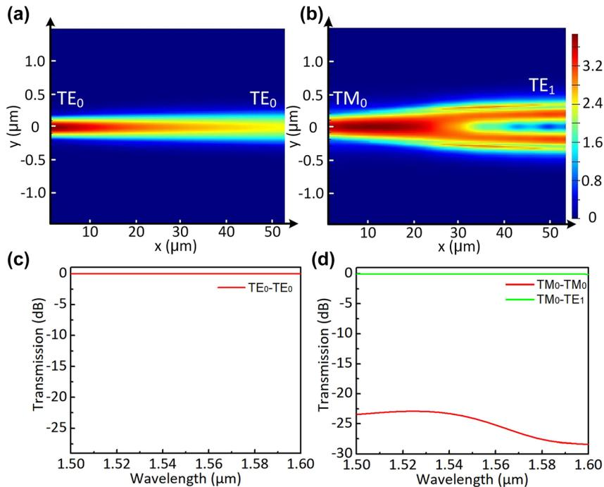
**Figure 3:** Simulated light propagation in the designed PDMC for the launched  $TE_0$  (a) and  $TM_0$  (b) modes with the FDTD method; and calculated transmission spectra in the designed PDMC for the launched  $TE_0$  (c) and  $TM_0$  (d) modes.
