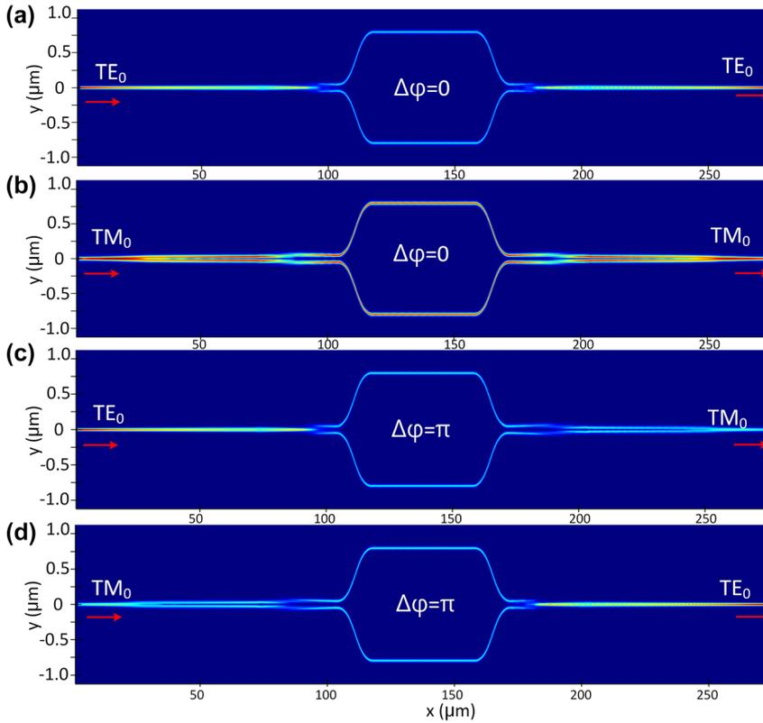
**Figure 7:** Simulated light propagation of the designed polarization switch for the launched  $TE_0$  (a) and  $TM_0$  (b) modes with  $\Delta\phi = 0$ ; simulated light propagation of the designed polarization switch for the launched  $TE_0$  (c) and  $TM_0$  (d) modes with  $\Delta\phi = \pi$ .
