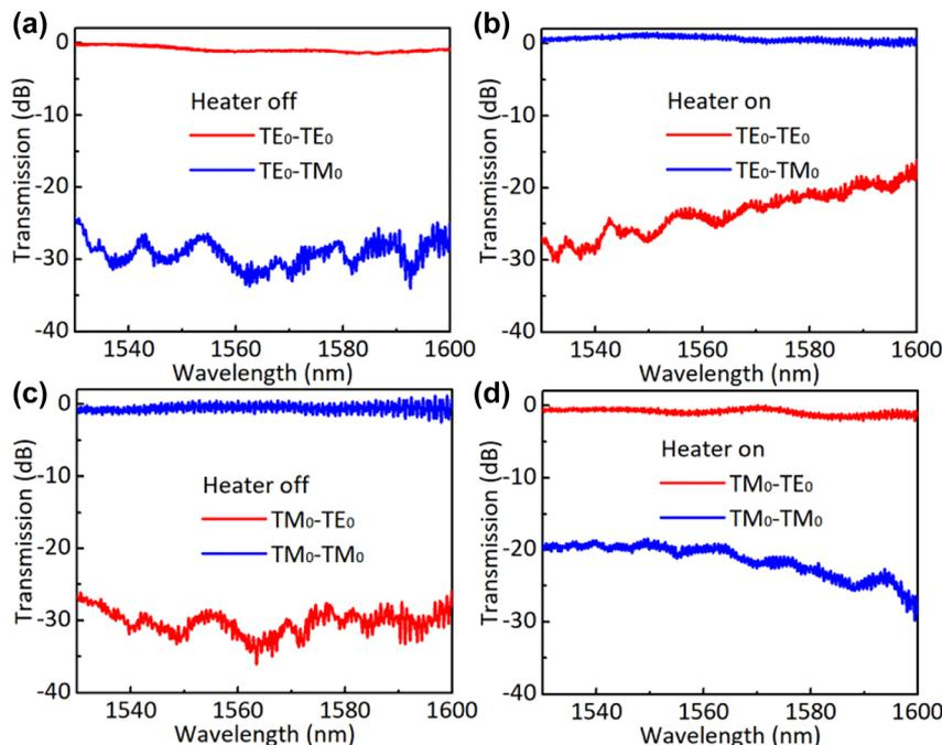
**Figure 10:** Measured transmissions of the fabricated polarization switch for the launched TE<sub>0</sub> (a) and TM<sub>0</sub> (b) modes when it is off; measured transmissions of the fabricated polarization switch for the launched TE<sub>0</sub> (c) and TM<sub>0</sub> (d) modes when it is on.
