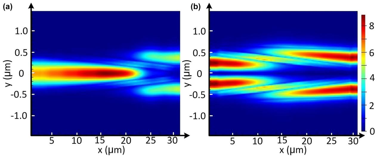
**Figure 5:** Simulated light propagation in the designed power splitter for the launched  $TE_0$  (a) and  $TE_1$  (b) modes.
