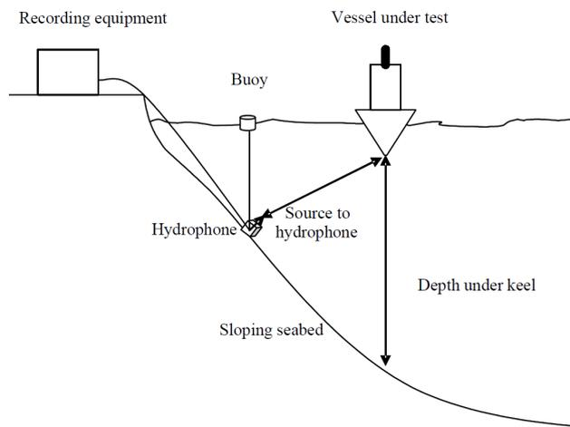
Figure 5: Sketch for underwater noise measurements (from [52]).
