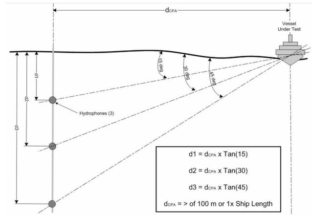
Figure 4: Sketch for underwater noise measurements (from [51]).
