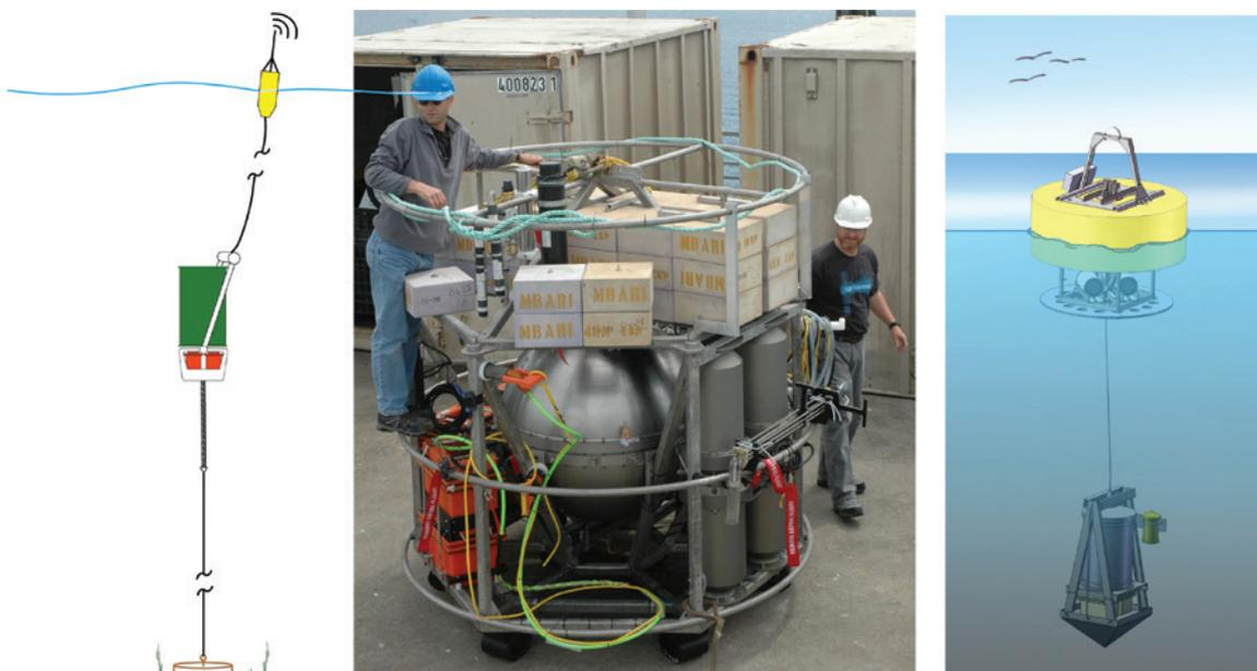
**Fig. 2:** Different mooring configurations allow access to different environments. A typical moored configuration (left) places the 2G-ESP up to 50 m deep, with communications via a buoy cell phone. A 1 m titanium sphere allows deployments to depths of 4000 m (middle) and communication via acoustic modem. A freely drifting configuration (right) can remain in the same parcel of (moving) water and collect samples over time.
