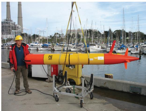
**Fig. 3:** The long-range autonomous underwater vehicle (LRAUV) with the 3G-ESP mounted in the forward yellow body section.
