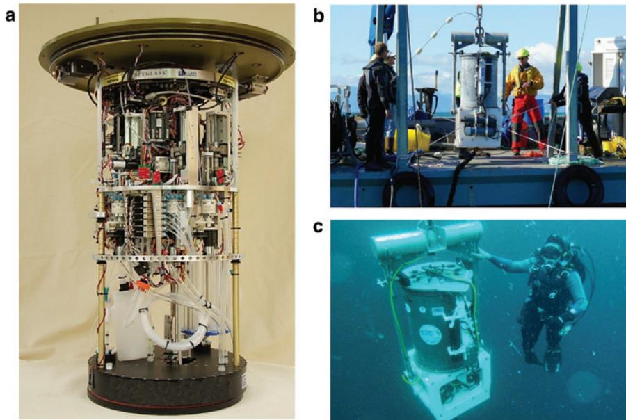
**Fig. 1:** The Environmental Sample Processor (ESP) is a self-contained, autonomous, robotic water sampler capable of performing several types of molecular biological assay in situ. (a) Instrument attached to pressure housing lid. (b) Deploying the ESP in a New Zealand shellfish farm. (c) ESP in surface mooring configuration with diver support.
