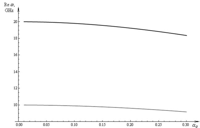
**Figure 4:** Dependence of  $\text{Re } \omega$  on  $\alpha_G$  for typical values of the nanotube parameters. The thinner line represents the dependence for  $k = 10^2$  cm<sup>-1</sup>, thick line – for  $k = 10^6$  cm<sup>-1</sup>.
