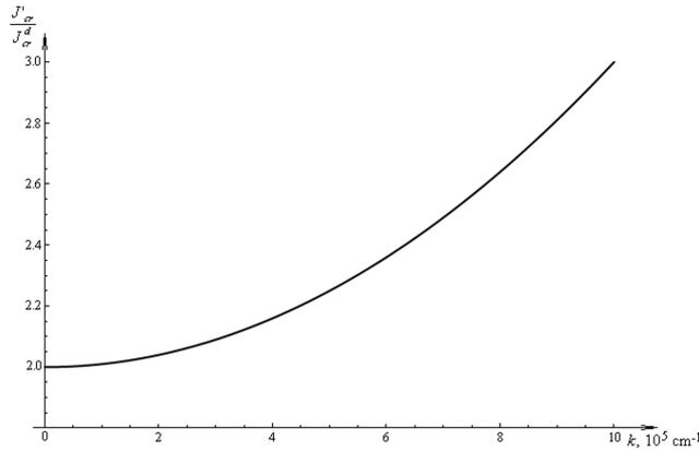
**Figure 6:** Relation of critical current for a nanotube to a critical current for a nanodisc for typical nanosystem parameters.
