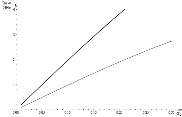
**Figure 5:** Dependence of  $\text{Im } \omega$  on  $\alpha_G$  for typical values of the nanotube parameters. The thinner line represents the dependence for  $k = 10^2 \text{ cm}^{-1}$ , thick line – for  $k = 10^6 \text{ cm}^{-1}$ .
