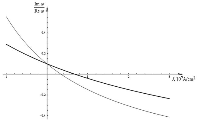
**Figure 3:** Dependence of  $\text{Im } \omega / \text{Re } \omega$  on  $J$  for typical values of the nanotube parameters. Thinner line represents the dependence for  $k = 10^2$  cm<sup>-1</sup>, thick line – for  $k = 10^6$  cm<sup>-1</sup>.
