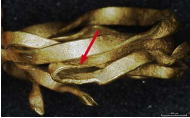
Fig. 5: Creases at the longitudinal edges as evidence of the flattening process of the wire (microscope image: Christoph Berthold, CCA Tübingen).
