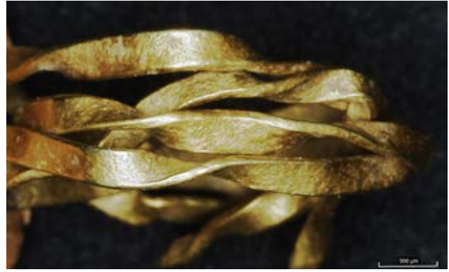
Fig. 6: The two strips twist differently (microscope image: Christoph Berthold, CCA Tübingen).
