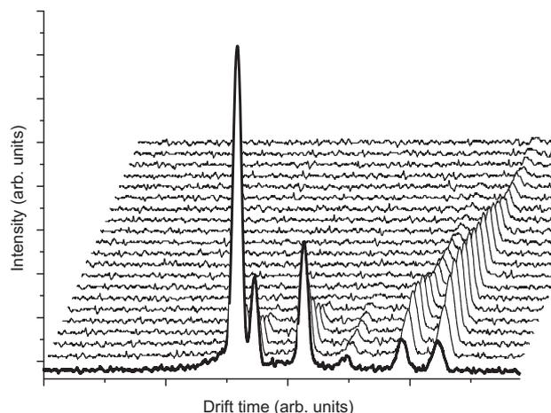
**Figure 2** Typical IMS spectrum, shown for a mixture of dimethyl methylphosphonate (DMMP) and dimethylformamide (DMF). The six peaks (from left to right) are RIP, DMF monomer, DMMP monomer, DMF dimer, DMMP+DMF asymmetric dimer, DMMP dimer. Furthermore, it is shown how the spectrum changes if a pulsed source is used and the delay time between ionizing electron pulse and ion extraction (with subsequent detection) is increased (each spectrum was recorded 300  $\mu$ s after the previous one).
