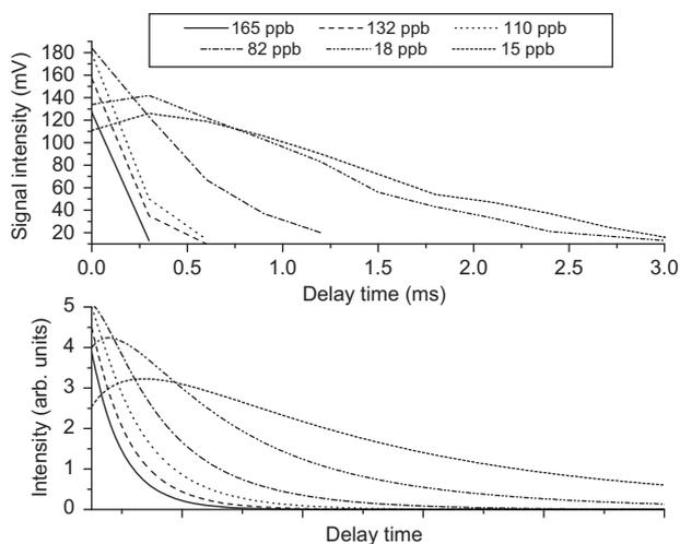
**Figure 5** Comparison of measured (upper graph) and calculated (lower graph) signal intensities for a monomer signal (measurements shown for ethyl methyl ketone).
