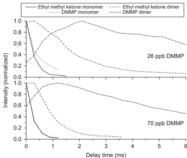
**Figure 6** Dimer and monomer signals decay differently in mixtures, here shown for DMMP and ethyl methyl ketone (concentration 110 ppb). The dimer signals decay much more slowly, and the dimer of the substance with the higher proton affinity (DMMP) decays most slowly even if its concentration is low compared to the other substance's concentration.
