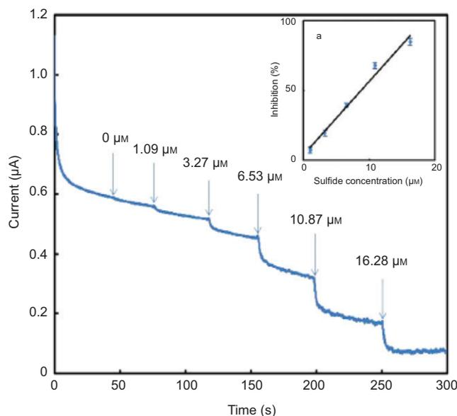
**Figure 2** Amperometric response of coprinus cinereus peroxidase (CIP) biosensor for different concentrations of sulfide at  $-150$  mV versus Ag/AgCl in 0.1 M phosphate buffer (pH 6.5) solution containing  $0.6 \text{ mM H}_2\text{O}_2$  and  $1.25 \text{ mM}$  of hydroquinone. Inset (A): calibration curve for sulfide determination with CIP inhibition sensor.
