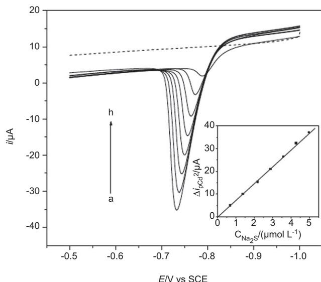
**Figure 1** The anodic stripping voltammetry (ASV) response of  $\text{Cd}^{2+}$  changed with the addition of sulfide. 0.1 M pH 4.5 NaAc-HAc (---base line) buffer solution at  $3.6 \times 10^{-6}$  M; A–H:  $C_{\text{S}^{2-}} = 0, 0.7, 1.4, 2.2, 2.9, 3.6, 4.3, 5.0 \times 10^{-6}$  M. Inset: plot of the relation between the peak current of  $\text{Cd}^{2+}$  and the concentration of sulfide added.
