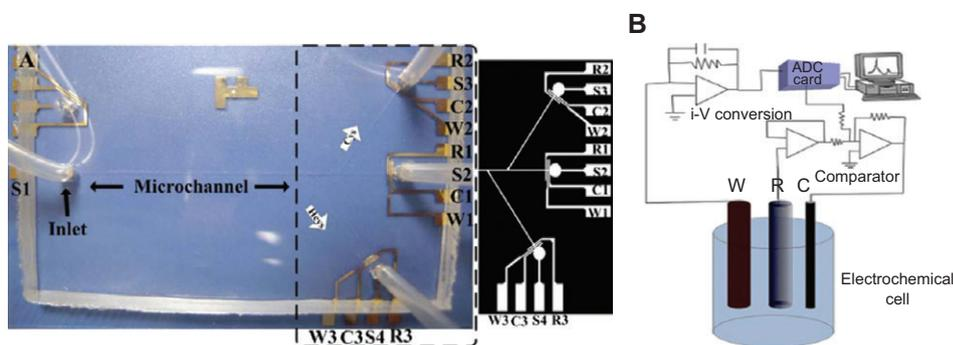
**Figure 5** (A) Image of capillary electrophoresis-amperometric detection (CE-AD) microchip showing microchannel engraved in polydimethylsiloxane (PDMS) mold, sample reservoirs, silicon tubes carrying sample and NaOH solution into the microchannel, gold microelectrodes (W1-3=working; C1-3=counter; R1-3=reference; S1-4=separation electrodes); and (B) schematics for electronic circuit and the operation of the in-house built dual potentiostat.
