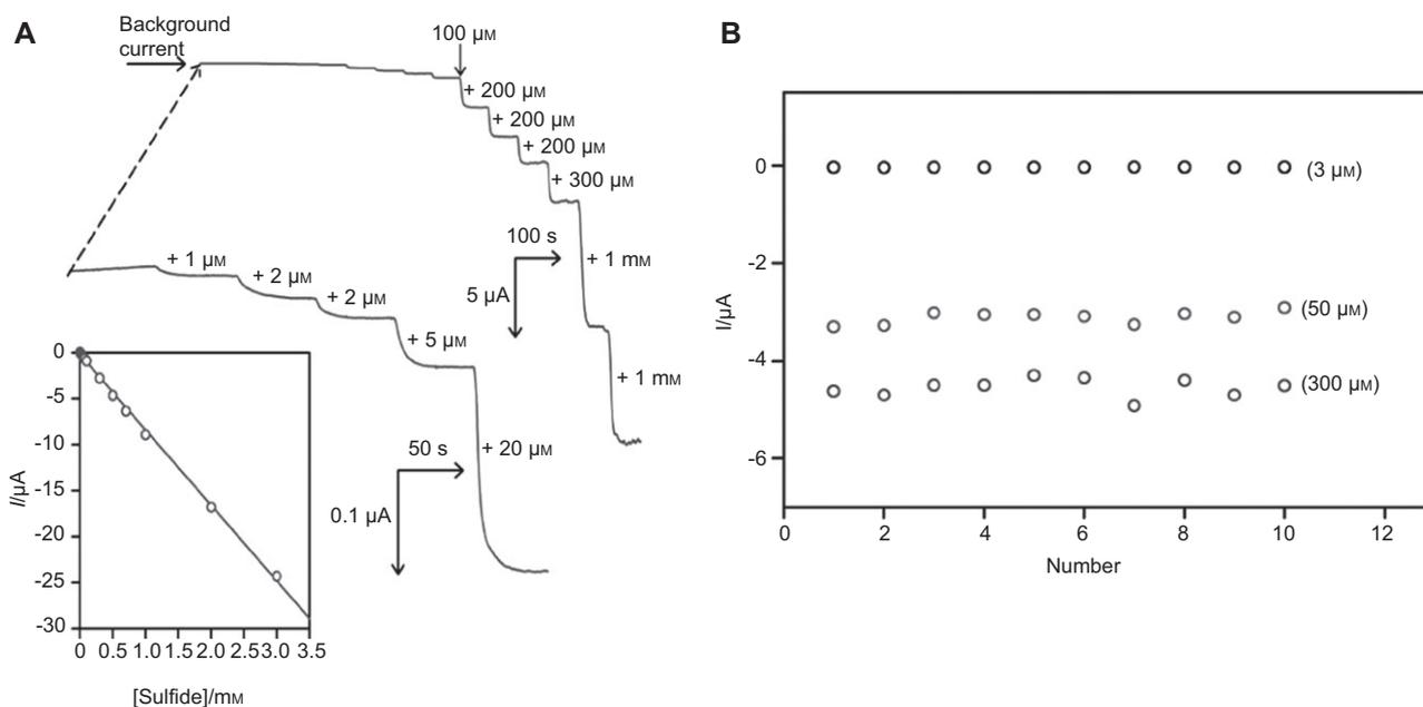
**Figure 3** (A) Chronoamperometric response of sulfide at the FeCN-PIL-SPCE in pH 7, 0.1 M PBS at a detection potential of 0.0 V versus Ag/AgCl. The insert graph is the calibration curve with a linear concentration range of 1  $\mu\text{M}$  to 3 mM; and (B) the results at the FeCN-PIL-SPCE for 10 continuous additions of 3  $\mu\text{M}$ , 50  $\mu\text{M}$  and 300  $\mu\text{M}$  sulfide, respectively.
