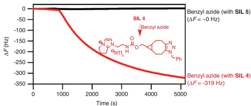
**Figure 4:** Chemoselective detection of benzyl azide gas (146 ppb) by 9 MHz QCM thin coated with **SIL 4** and **SIL 5** (3.3 nl each, 300 nm thickness).
