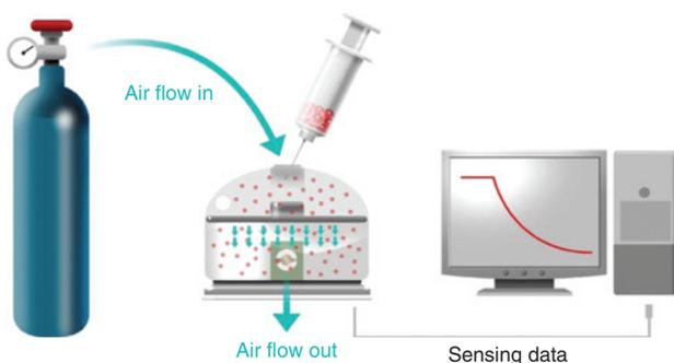
**Figure 2:** Schematic representation of a SIL-on-QCM gas analysis system for chemoselective gas sensing by specific chemical reactions.
