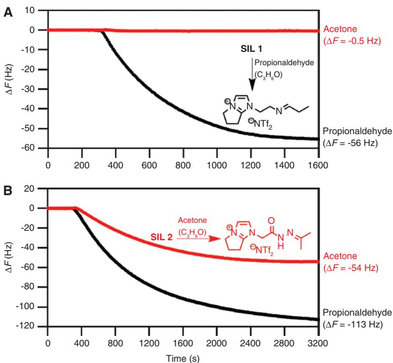
**Figure 3:** Chemoselective detection of acetone and propionaldehyde gases (98 ppb each) of identical molecular weight ( $\text{C}_3\text{H}_6\text{O}$ ) by 9 MHz QCM thin coated with (A) **SIL 1** and (B) **SIL 2** (3.3 nl each, 300 nm thickness).
