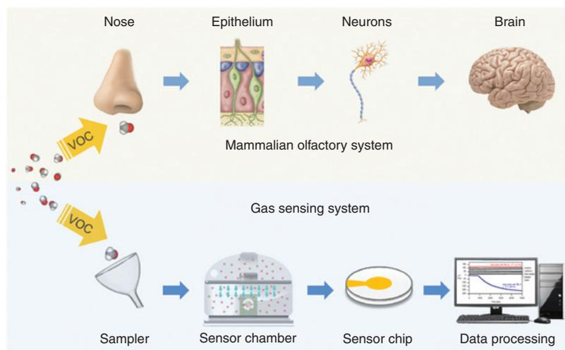
**Figure 1:** Schematic comparison of mammalian olfactory system and the QCM gas sensing system.
