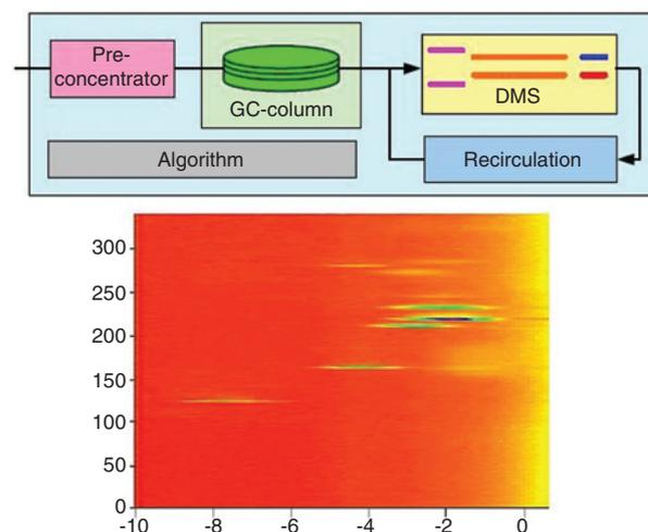
Figure 1: Instrumental implementation of GC-DMS MicroAnalyzer™.
