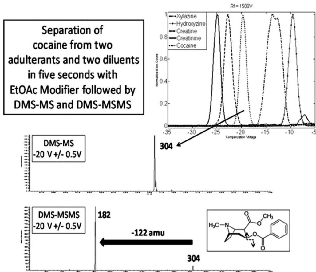
Figure 5: Detection of four additives and cocaine by DMS-MS.
