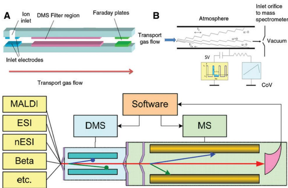
Figure 3: Schematic of DMS-MS principles and interface operation.
