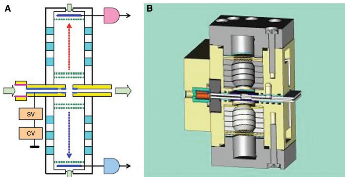
Figure 7: Schematic of DMS-IMS<sup>2</sup>.
