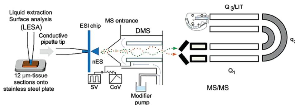
Figure 6: Detection platforms for LESA-DMS-MS/MS analyses.
