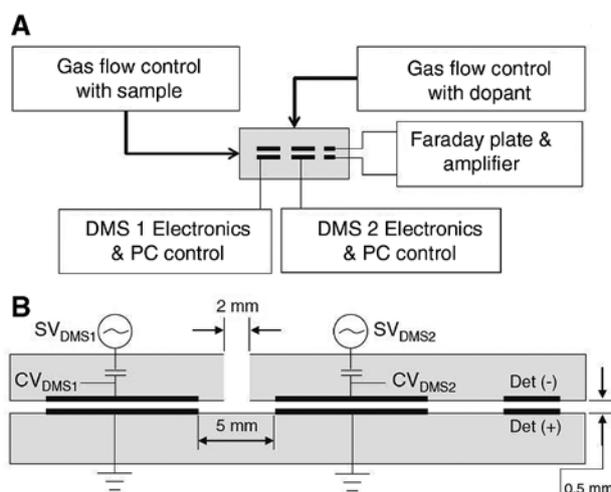
Figure 8: Schematic of a DMS/DMS system with enlarged graphics of the DMS/DMS analyzer.
