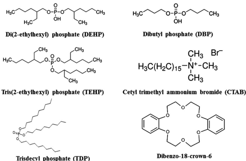
Figure 4: Structures for the representatives of additives in EME.
