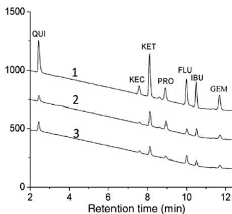
**Figure 2:** Sample clean-up capability of EME: chromatograms of the acceptor solutions after 20-min EME from 40 times diluted plasma (1) and after 10-min EME from 6 times diluted plasma (2), and the standard solution (3) (STD, 5  $\mu\text{g}/\text{ml}$ ). Reprinted from Ref. Huang et al. 2015f, with permission © 2015 Elsevier B.V.
