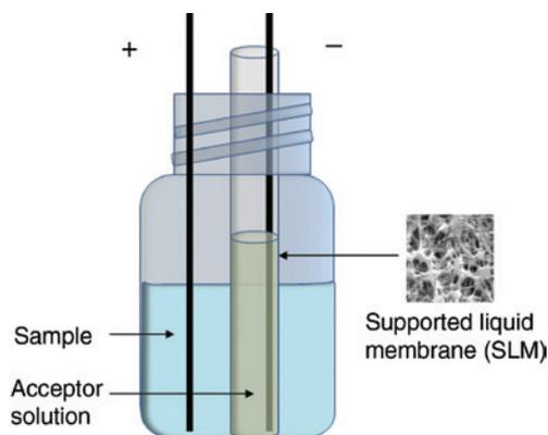
**Figure 1:** Schematic illustration of electromembrane extraction (EME) with hollow fiber membrane.
