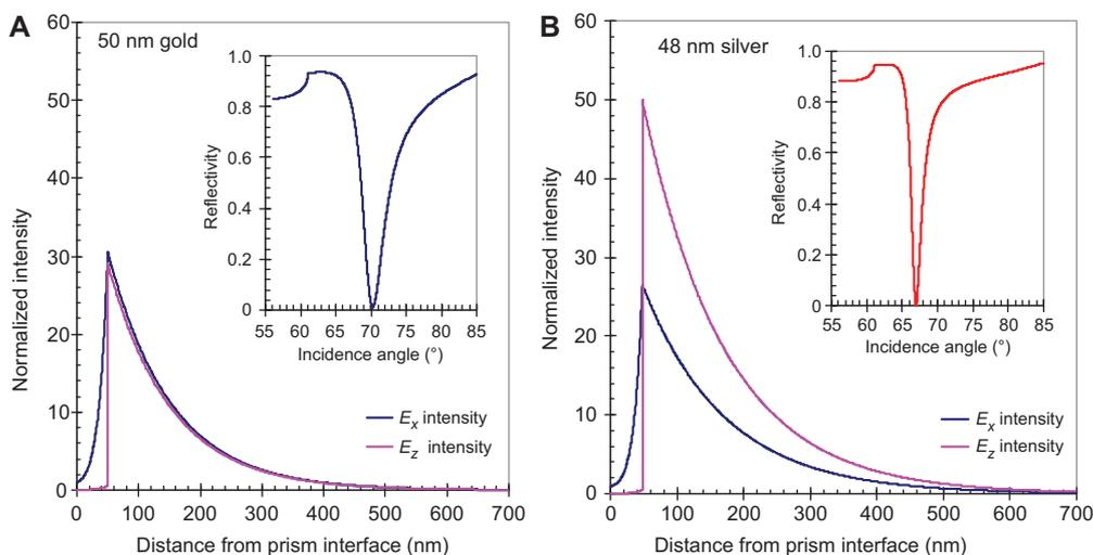
**Figure 4** Electromagnetic field intensity distributions with increasing distance from the prism interface using Kretschmann configuration for: (A) 50 nm gold; and (B) 48 nm silver films.  $E_x$  (blue) and  $E_z$  (pink): parameters used for calculations:  $n_{prism}=1.52$ ,  $\lambda=670$  nm,  $n_{analyte}=1.33$ . The insets present the reflectivity profiles for both cases.
