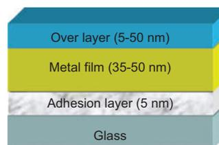
**Figure 1** Schematic illustration of SPR lamellar structure of dielectric-on-gold substrate.
