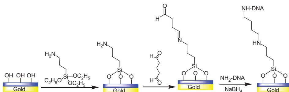
**Figure 8** Schematic outline of the covalent linking of amine-terminated bioreceptors to silica coated SPR interfaces.
