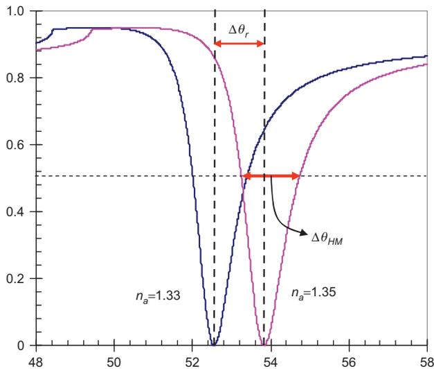
**Figure 3** Change in surface plasmon resonance signal due to a change in the analyte refractive index:  $n_a=1.33$  (blue),  $n_a=1.35$  (pink).
