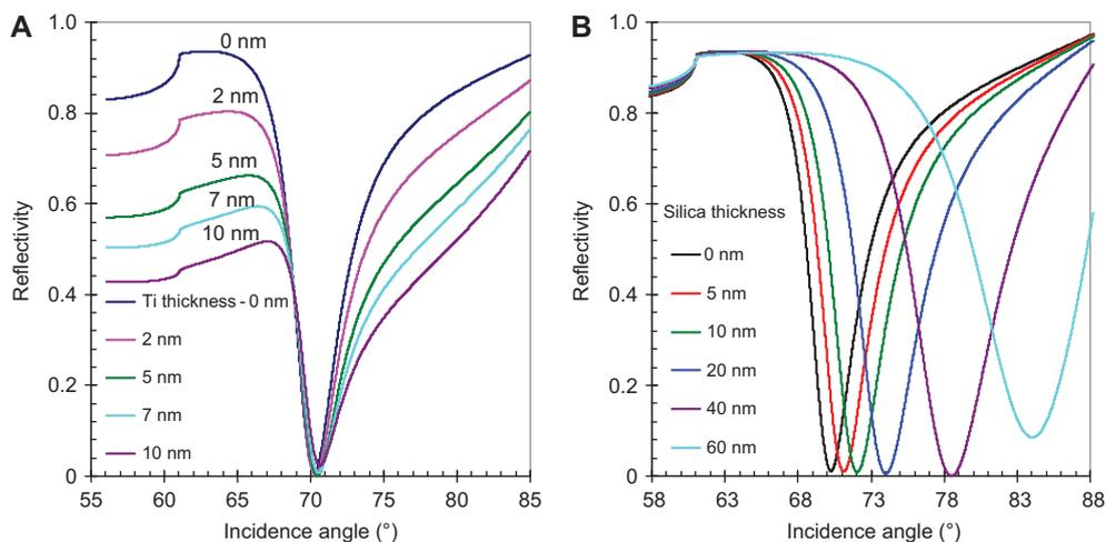
**Figure 5** Influence of: (A) Ti adhesion layer between glass prism and metal film; and (B) silica top layer of different thickness on performances of SPR sensor; parameters used for calculations:  $n_{prism}=1.52$ ,  $\lambda=670$  nm,  $n_{analyte}=1.33$ ,  $d_{gold}=50$  nm,  $n_{silica}=1.48$ ,  $d_{silica}=0-60$  nm,  $n_{titanium}=2.32+3.08i$ ,  $d_{Ti}=0-10$  nm.
