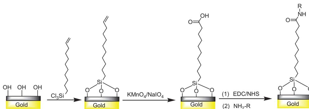
**Figure 11** Schematic illustration of the carboxylation of oxide-based overlayers such as ITO and  $\text{SnO}_2$ :Sb.
