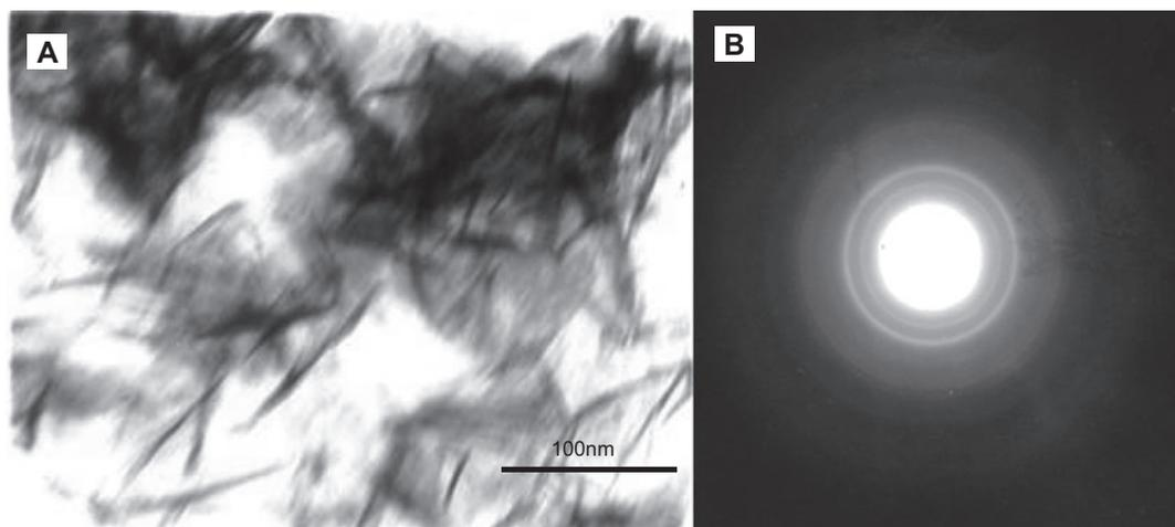
**Figure 3** (A) TEM photo of HAp/Col-48 composite; (B) electron diffraction graphic of HAp/Col-48 composite.
