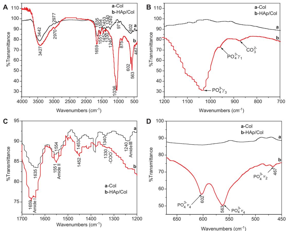
**Figure 4** Comparative analysis of FT-IR spectra of Col and HAp/Col. (A) Spectrum for wavelength range of 400–4000  $\text{cm}^{-1}$ ; (B) zoom-in spectrum for wavelength range of 700–1200  $\text{cm}^{-1}$ ; (C) zoom-in spectrum for wavelength range of 1200–1700  $\text{cm}^{-1}$ ; (D) zoom-in spectrum for wavelength range of 450–670  $\text{cm}^{-1}$ .
