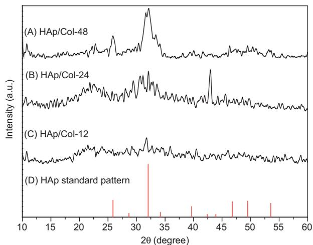
**Figure 1** XRD patterns of HAp/Col composites with varied aging time: (A) 48 h; (B) 24 h; (C) 12 h; (D) HAp standard pattern.
