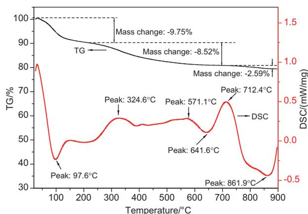
**Figure 5** TG and DSC plot of as-prepared HAp/Col composite.
