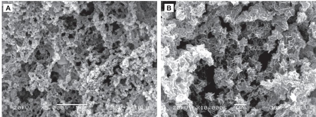
**Figure 2** SEM images of as-prepared HAp/Col composite (sample HAp/Col-48). (A) Surface morphology with a lower magnification; (B) cross-sectional fracture morphology at a higher magnification.
