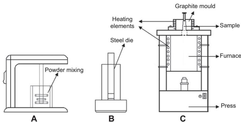
**Figure 1** Schematic illustration of the thixomoulding unit used for the production of MMCs (A) the mixture of A356 alloy and SiC<sub>p</sub> powder. (B) Preshaping of powder by cold pressing, and (C) the application of the semisolid process.
