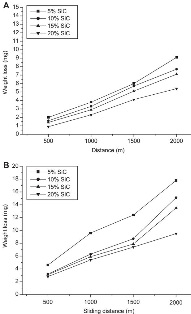
**Figure 3** The weight losses of the MMCs produced at 590°C (A) and 600°C (B).
