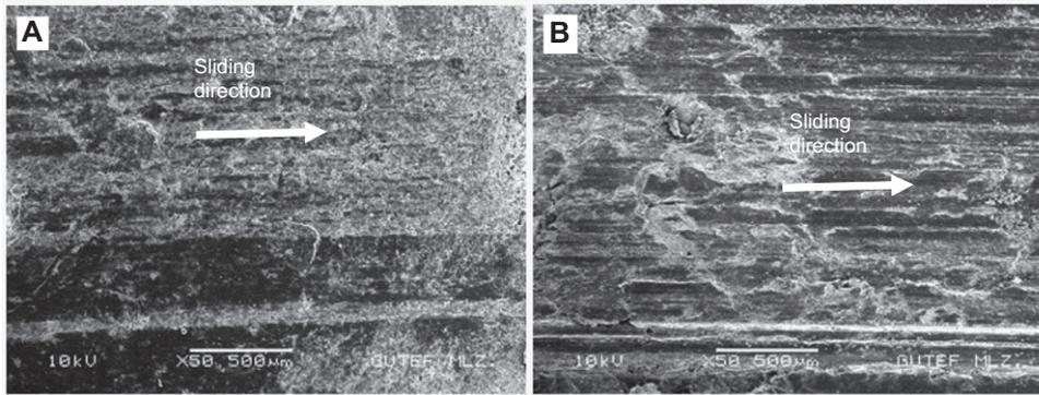
**Figure 5** The wear surface SEM images of the MMCs containing 20 vol.% of SiC and produced at 590°C (A) and 600°C (B) through semisolid processing.
