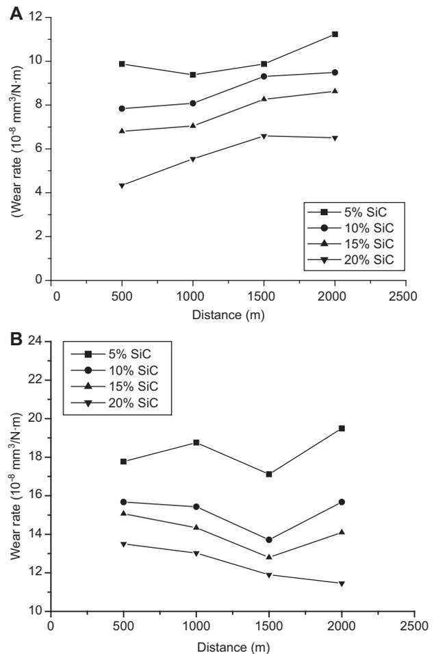
**Figure 4** The wear rates of the MMCs produced at 590°C and 600°C.
