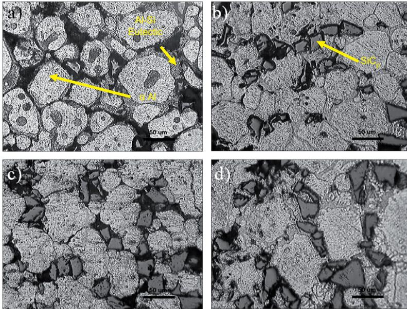
**Figure 2** The optical microscope images of MMC materials reinforced with SiC<sub>p</sub> at the rate of 590°C (a) 5%, (b) 10%, (c) 15% and (d) 20%.
