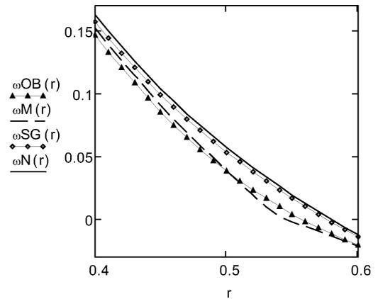
Fig. 4. Profiles of the velocity  $w(r,t)$  for Oldroyd-B, Maxwell, second-grade, and Newtonian fluids, for  $\nu = 0.003$ ,  $\mu = 2.916$ ,  $R_1 = 0.4$ ,  $R_2 = 0.6$ ,  $f = -5$ ,  $\lambda = 4$ ,  $\lambda_r = 1$ , and  $t = 5$  s.
