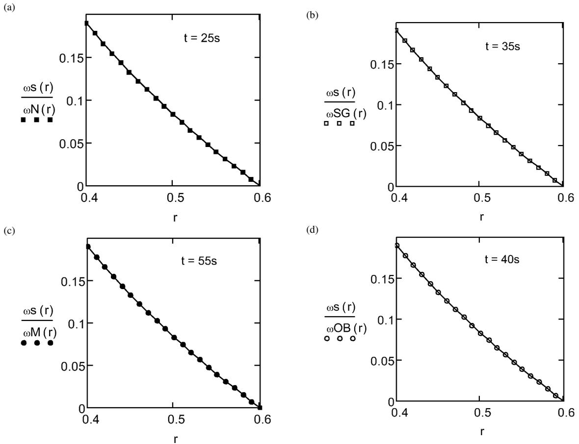
Fig. 5. Required time to reach the steady-state for Newtonian, second-grade, Maxwell, and Oldroyd-B fluids, for  $\nu = 0.003$ ,  $\mu = 2.916$ ,  $R_1 = 0.4$ ,  $R_2 = 0.6$ ,  $f = -5$ ,  $\lambda = 3$ , and  $\lambda_r = 1$ .
