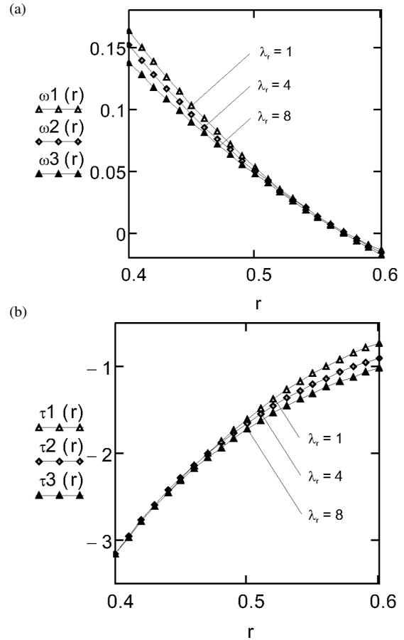
Fig. 3. Profiles of the velocity  $w(r,t)$  given by (17) and shear stress  $\tau(r,t)$  given by (19), for  $\nu = 0.003$ ,  $\mu = 2.916$ ,  $R_1 = 0.4$ ,  $R_2 = 0.6$ ,  $f = -5$ ,  $\lambda = 10$ ,  $t = 10$  s and different values of  $\lambda_r$ .
