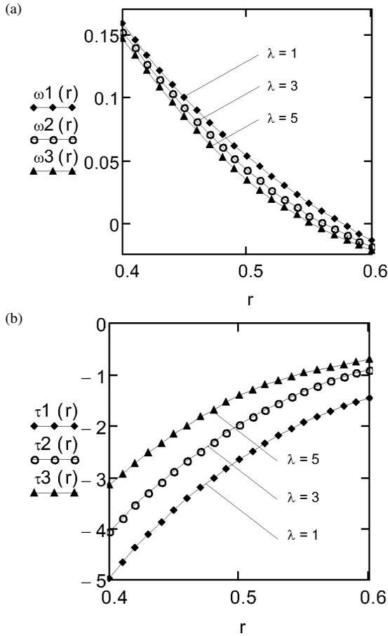
Fig. 2. Profiles of the velocity  $w(r,t)$  given by (17) and shear stress  $\tau(r,t)$  given by (19), for  $\nu = 0.003$ ,  $\mu = 2.916$ ,  $R_1 = 0.4$ ,  $R_2 = 0.6$ ,  $f = -5$ ,  $\lambda_r = 0.5$ ,  $t = 5$  s and different values of  $\lambda$ .
