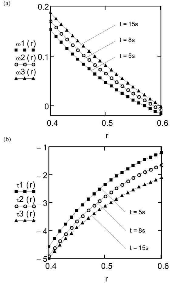
Fig. 1. Profiles of the velocity  $w(r,t)$  given by (17) and shear stress  $\tau(r,t)$  given by (19), for  $\nu = 0.003$ ,  $\mu = 2.916$ ,  $R_1 = 0.4$ ,  $R_2 = 0.6$ ,  $f = -5$ ,  $\lambda = 2$ ,  $\lambda_r = 1$ , and different values of  $t$ .
