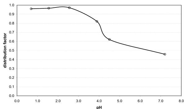
Fig. 2. Dependence of distribution coefficient on pH value for P(3-py)<sub>3</sub> in cyclohexane/water.
