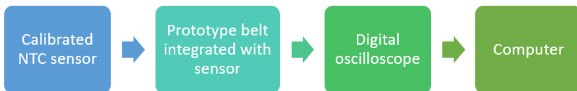
Figure 1. Scheme of the setup used as a temperature monitoring system.
