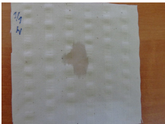
Figure 12. Spreading the liquid moisture on the flat and puckered surface of the seersucker fabric
