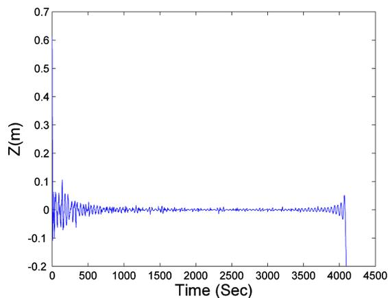
Figure 12. Heights of moored-sea GPS buoy after filtering.
