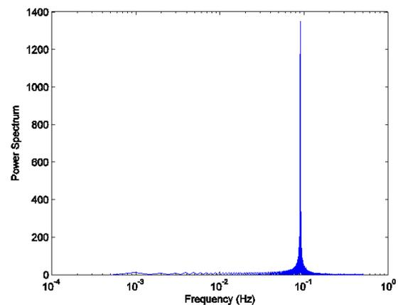
Figure 4. Power spectrum of the heaved wave data from the wave simulator in the laboratory experiment (in  $m^2/Hz$ ).
