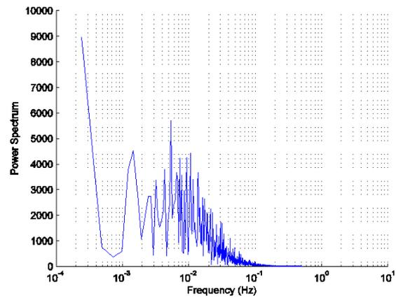
Figure 2. Power spectrum of the GPS height data from the wave simulator collected during the laboratory experiment (in  $m^2/Hz$ ).
