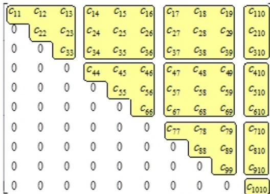
Figure 1. Chunk-wise division of the upper-triangular part of the  $\bar{C}$  matrix concatenated contingently with the parameter matrix  $A$ . Each element  $c_{ij}$  is a sub-matrix of size  $k \times k$ . In the figure a chunk consist of  $3 \times 3$  blocks.
