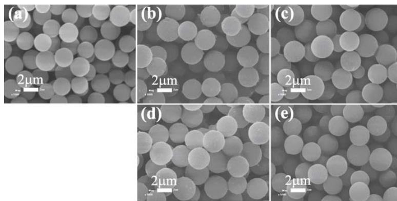
**Figure 1.** SEM images of the “living” core polymer microspheres (a), the ungrafted CS-MIP (b)/CS-CP (c) microspheres, and the grafted CS-MIP (d)/CS-CP (e) microspheres. The scale bar is 2  $\mu\text{m}$  in the above images.
