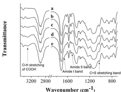
**Figure 2.** FT-IR spectra of the "living" core polymer microspheres (a), the ungrafted CS-MIP (b)/CS-CP (c) microspheres, and the grafted CS-MIP (d)/CS-CP (e) microspheres.
