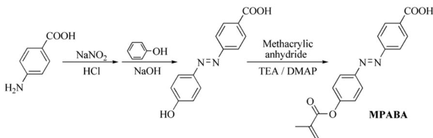
Scheme S1. Synthetic route to azobenzene functional monomer 4-((4-methacryloyloxyphenyl)azobenzoyl)benzoic acid (MPABA).
