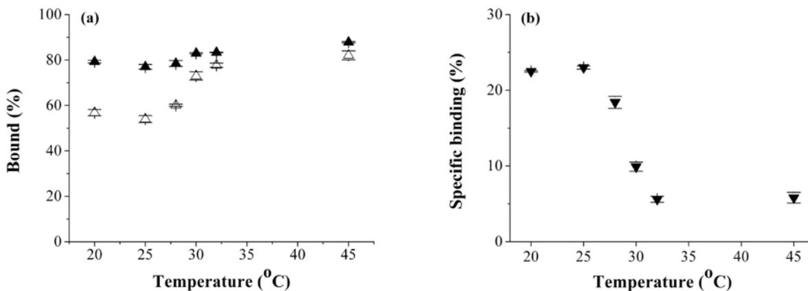
Figure S6. (a) Temperature-dependent equilibrium bindings (as percentage values) of the grafted CS-MIP (filled triangle)/CS-CP (open triangle) microspheres towards propranolol in real water; (b) Temperature-dependent specific bindings (as percentage values) of the grafted CS-MIP microspheres towards propranolol in real water: Polymer concentration = 1.0 mg/mL,  $C_{\text{propranolol}} = 0.05 \text{ mM}$  (the binding analyses were performed in duplicate).
