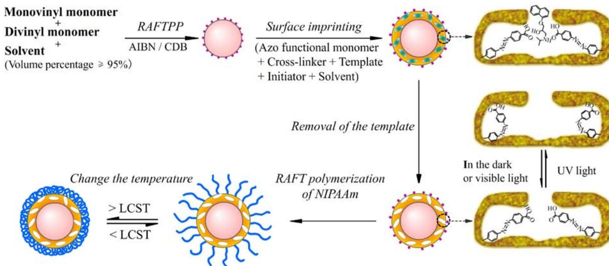
**Scheme 1.** Synthesis of narrowly dispersed MIP microspheres with both photo- and thermo-responsive template binding properties in pure aqueous media by RAFT polymerization and their stimuli-responsive behavior.
