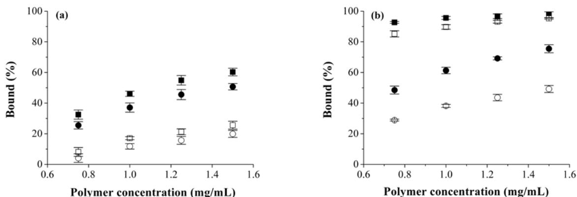
**Figure 3.** Equilibrium bindings (as percentage values) of propranolol on different amounts of the ungrafted (square) and grafted (circle) CS-MIP (filled symbols)/CS-CP (open symbols) microspheres in its solution (0.05 mM) in acetonitrile (a) and in pure water (b) at 25°C, respectively (the binding analyses were performed in duplicate).
