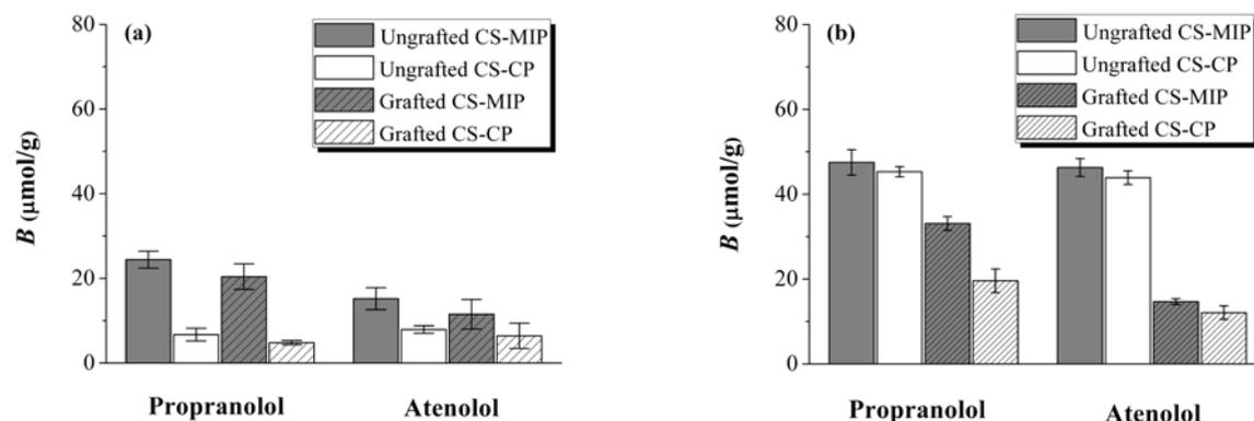
**Figure 4.** Selective bindings of the ungrafted and grafted CS-MIP/CS-CP microspheres towards propranolol and atenolol in their mixed solution ( $C_{\text{Propranolol or atenolol}} = 0.05 \text{ mM}$ ) in acetonitrile (a) and in pure water (b), respectively (polymer concentration: 1 mg/mL) (the binding analyses were performed in duplicate).
