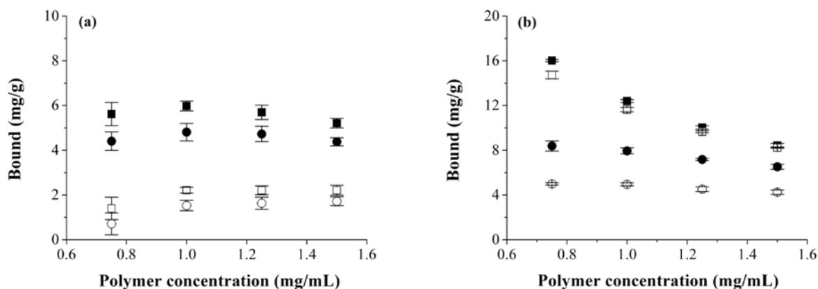
Figure S1. Equilibrium bindings (as mg template per gram polymer microspheres) of propranolol on different amounts of the ungrafted (square) and grafted (circle) CS-MIP (filled symbols)/CS-CP (open symbols) microspheres in its solution (0.05 mM) in acetonitrile (a) and in pure water (b) at 25°C, respectively (the binding analyses were performed in duplicate).
