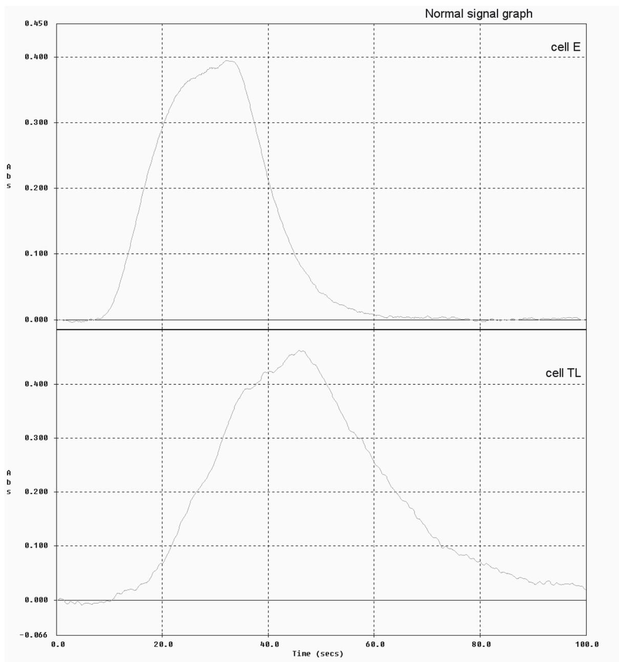
**Figure 6.** Time dependence of absorbance signal for cells **E** and **TL** in FIA mode:  $I = 0.7$  A (cell **E**) or  $1.2$  A (cell **TL**),  $v_{Ac} = 20.0$  mL  $\text{min}^{-1}$ ,  $v_{el} = 2.0$  mL  $\text{min}^{-1}$ ,  $c_{Se} = 100$   $\mu\text{g dm}^{-3}$ ,  $c_{el} = 1$  mol  $\text{dm}^{-3}$ , injected volume  $1000$   $\mu\text{L}$ .
