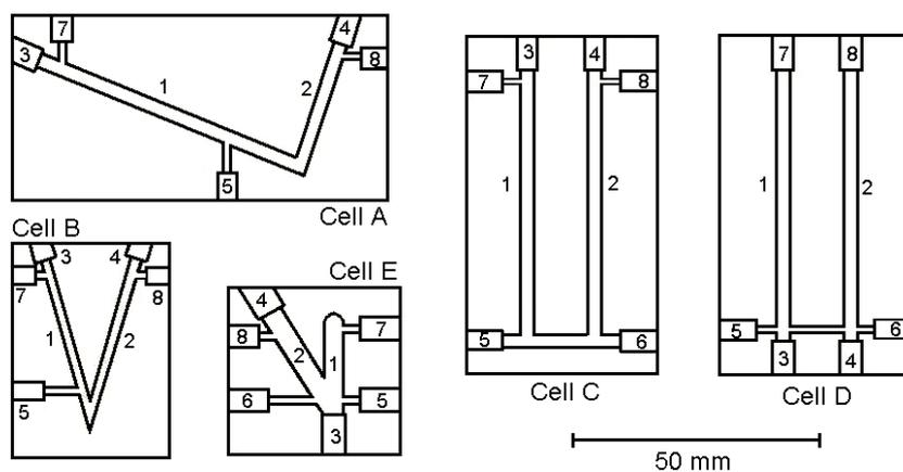
**Figure 1.** New flow-through electrolytic cells: 1 – cathode chamber, 2 – anode chamber, 3 – cathode holder, 4 – anode holder, 5, 6 – electrolyte inlet (pure or containing analyte), 7 – outlet to gas-liquid separator, 8 – waste outlet.
