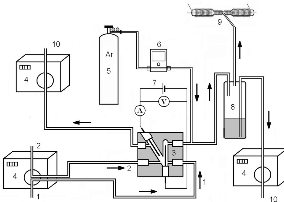
**Figure 2.** Instrumental setup for ECHG-QFAAS with cell **E**: 1 – catholyte, 2 – anolyte, 3 – flow-through electrolyte cell (type E), 4 – peristaltic pump, 5 – carrier gas, 6 – mass flow controller, 7 – electric current supply, 8 – gas-liquid separator, 9 – quartz tube atomizer, 10 – waste
