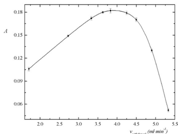
**Figure 3.** The dependence of the absorption signal on withdrawal flow rate for cell **D**:  $I = 0.25 \text{ A}$ ,  $v_{\text{Ar}} = 10 \text{ mL min}^{-1}$ ,  $v_{\text{el}} = 2.0 \text{ mL min}^{-1}$ ,  $c_{\text{el}} = 1 \text{ mol dm}^{-3}$ ,  $c_{\text{Se}} = 60 \mu\text{g dm}^{-3}$ .
