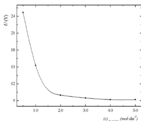
**Figure 5.** The dependence of the applied electric voltage on electrolyte concentration for cell **D**:  $I = 0.3 \text{ A}$ ,  $v_{\text{Ar}} = 10.0 \text{ mL min}^{-1}$ ,  $v_{\text{el}} = 2.5 \text{ mL min}^{-1}$ ,  $v_{\text{od}} = 3.8 \text{ mL min}^{-1}$ ,  $c_{\text{Se}} = 60 \mu\text{g dm}^{-3}$ .
