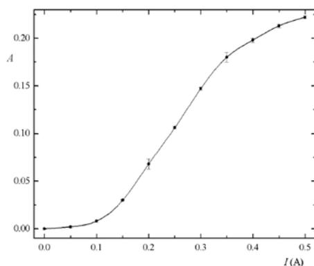
**Figure 4.** The dependence of absorption signal on the generation current for cell **B**:  $C_{\text{el}} = 1 \text{ mol dm}^{-3}$ ,  $v_{\text{Ar}} = 10 \text{ mL min}^{-1}$ ,  $v_{\text{el}} = 2.5 \text{ mL min}^{-1}$ ,  $c_{\text{Se}} = 60 \mu\text{g dm}^{-3}$ .
