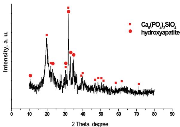
**Figure 7.** XRD of collagen-silicocarnotite (25:75 wt%) after 3 days immersion in 1.5 SBF
