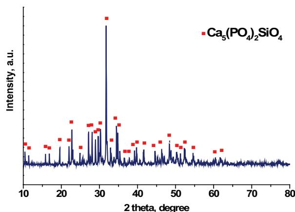
**Figure 1.** XRD patterns for silica containing sample, thermal treated at  $1200^\circ\text{C} / 2$  h
