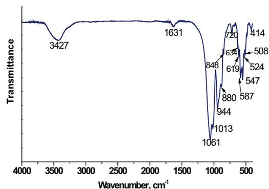
**Figure 2.** FTIR spectrum of silicocarnotite, heat treated at  $1200^\circ\text{C} / 2$  h
