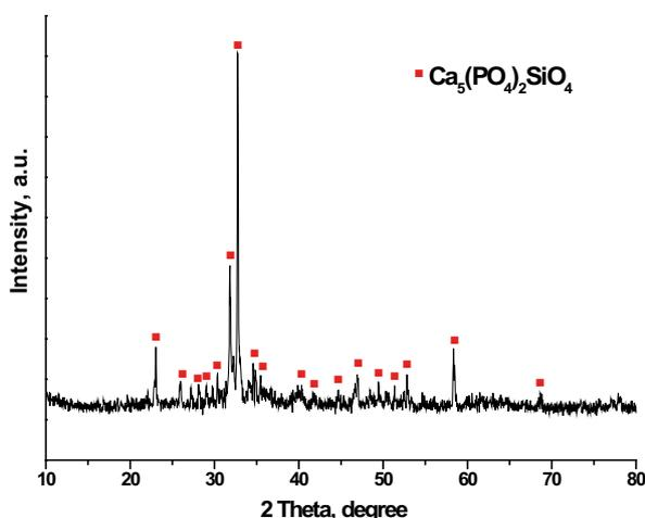
**Figure 5.** XRD of collagen/silicocarnotite (25:75 wt%) before immersion in 1.5 SBF
