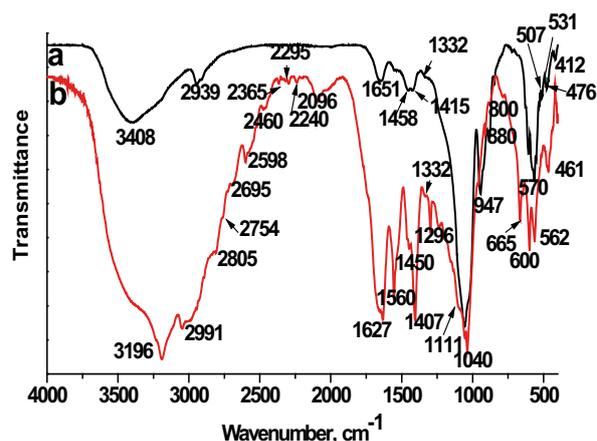
**Figure 6.** FTIR spectra of collagen/silicocarnotite coatings, after immersion in 1.5 SBF with different quantity of collagen and silicocarnotite: 25:75 wt.% (a) and 75:25 wt.% (b)
