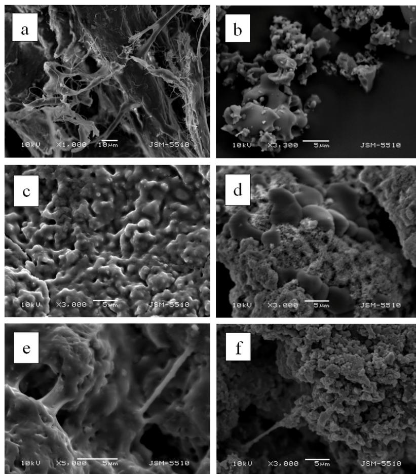
**Figure 8.** SEM images for pure collagen (a), silicocarnotite (b), silicocarnotite/collagen 75:25 wt% (c), silicocarnotite/collagen 25:75 wt% before SBF (d), silicocarnotite /collagen 75:25 wt% (e), silicocarnotite /collagen 25:75 wt% after immersion in SBF for 3 days (f)
