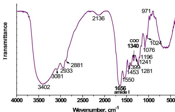
**Figure 3.** FTIR spectrum of pure collagen (Fluka)
