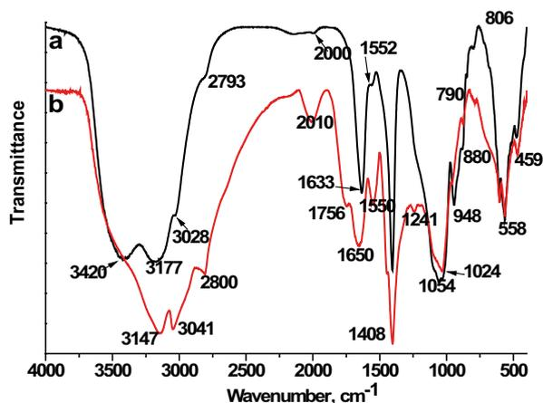
**Figure 4.** FTIR spectra of collagen/silicocarnotite coatings, before immersion in 1.5 SBF with different quantity of collagen and silicocarnotite: 25:75 wt% (a) and 75:25 wt% (b)
