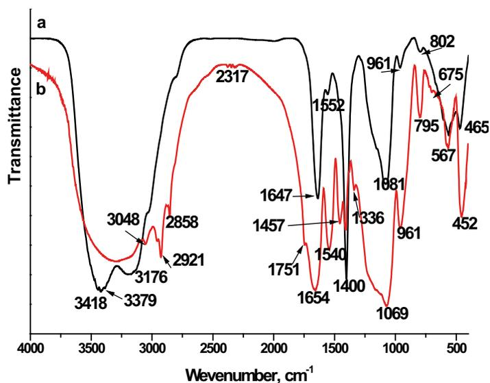
**Figure 4.** FTIR spectra of C-CPS/W hybrids with different quantity of C and CPS/W- 25:75 wt.% (a) and 75:25 wt.% (b), after 3 days immersion in 1.5 SBF
