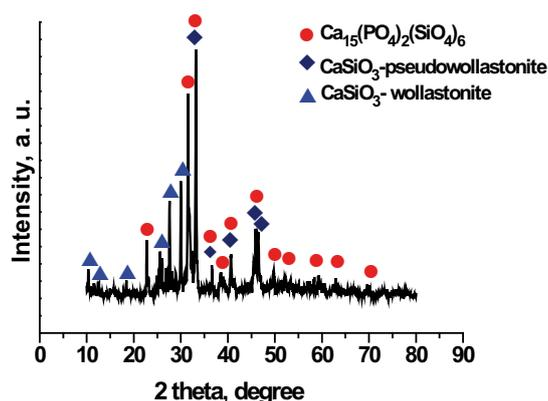
**Figure 1.** XRD patterns for the obtained calcium phosphate silicate, annealed at 1200°C/2 h
