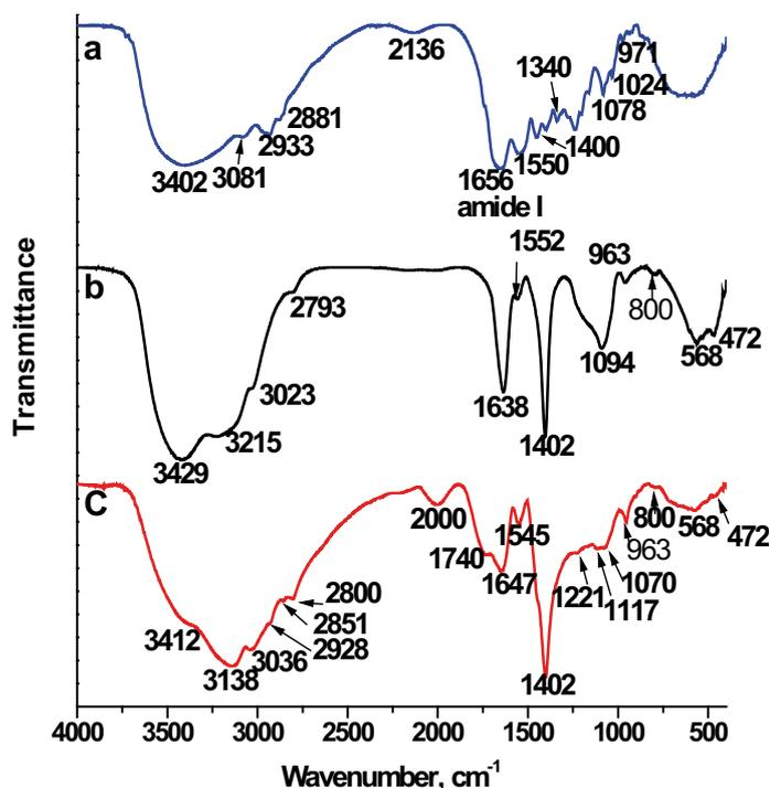
**Figure 3.** FTIR spectra of pure collagen (a), C-CPS/W-25:27 wt.% (b) and C-CPS/W-75:25 wt.% (c)
