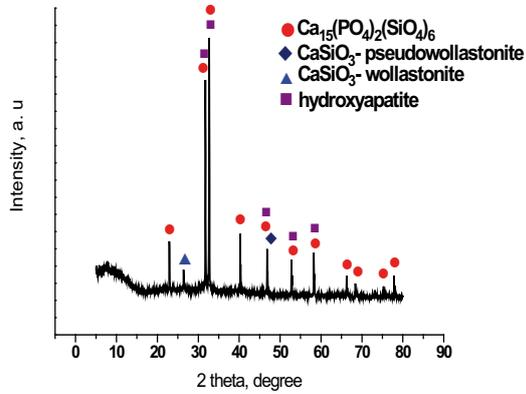
**Figure 5.** XRD of C-CPS/W (25:75 wt.%) after immersion in 1.5 SBF
