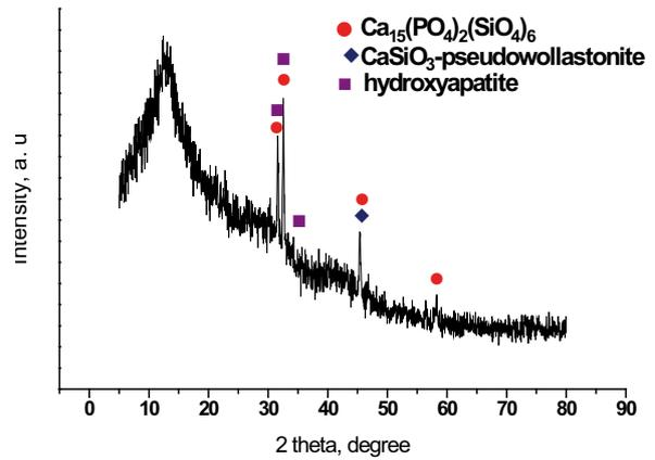
**Figure 6.** XRD of C-CPS/W (75:25 wt.%) after immersion in 1.5 SBF
