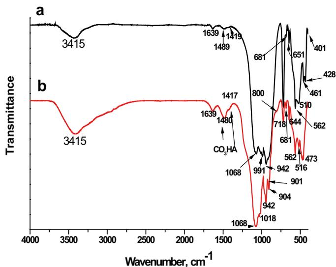
**Figure 2.** FTIR spectra of CPS/W thermal treated at 1200°C/2 h (a) and after immersion in TRIS-HCl buffer for 3 days (b)
