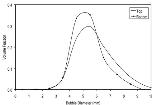
**Figure 6.** A comparison between bubble size distribution in term of volume fraction in bottom and top of column experimentally obtained for butanol solution.
