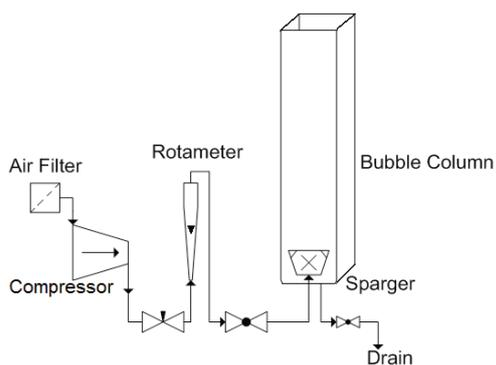
**Figure 3.** A schematic of the setup and bubble column used in the study.
