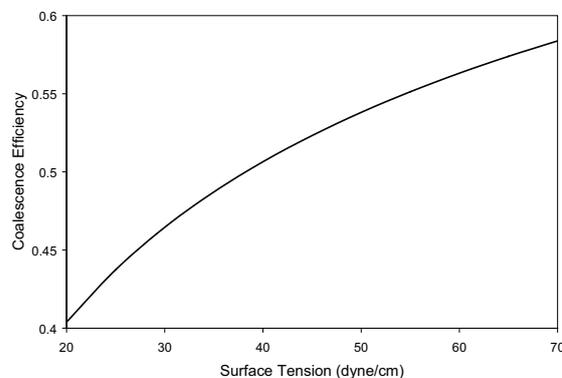
**Figure 4.** Coalescence efficiency vs. surface tension, plotted for a bubble of 0.5 mm in diameter in touch with a bubble of 5 mm in diameter.
