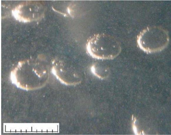
**Figure 1.** Formation of bubble bunch in the system containing air and butanol solution in water within a bubble column. Tiny bubbles attached to larger bubbles in the middle of picture are obvious. Scale shown on the bottom left is 10 mm.
