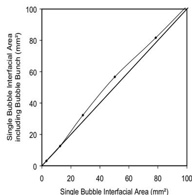
**Figure 7.** Interfacial area considering bubble bunch effect vs. interfacial area neglecting bubble bunch effect.
