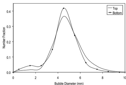
**Figure 5.** A comparison between bubble size distribution in term of number fraction in bottom and top of column experimentally obtained for butanol solution.
