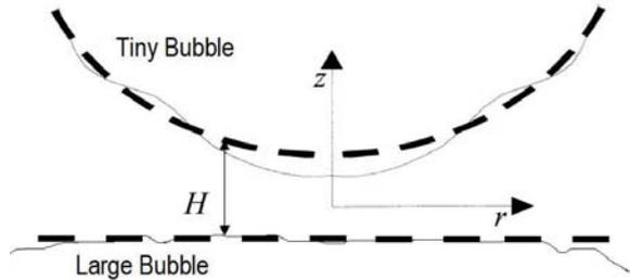
**Figure 2.** A sketch of a tiny bubble adjacent to a large bubble.
