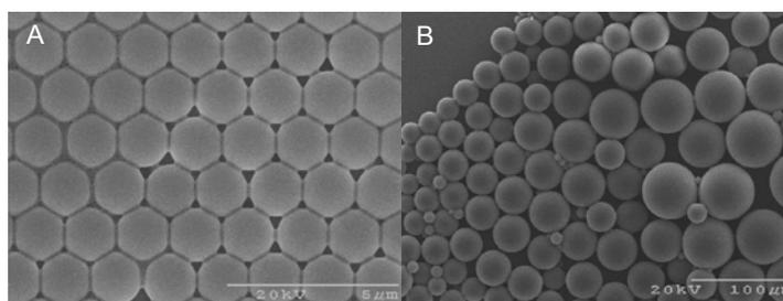
**Figure 3.** Scanning electron microscopic images of polystyrene particles prepared by (A) one-batch reverse ATRP and (B) two-stage reverse ATRP, respectively [123]. Reproduced with permission from the American Chemical Society.
