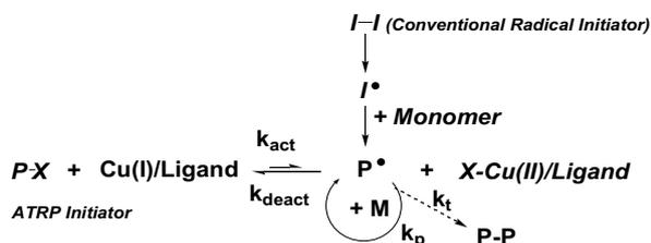
**Scheme 5.** Proposed mechanism for SR&NI process in ATRP. All ingredients present in the initial system are highlighted in italics.
