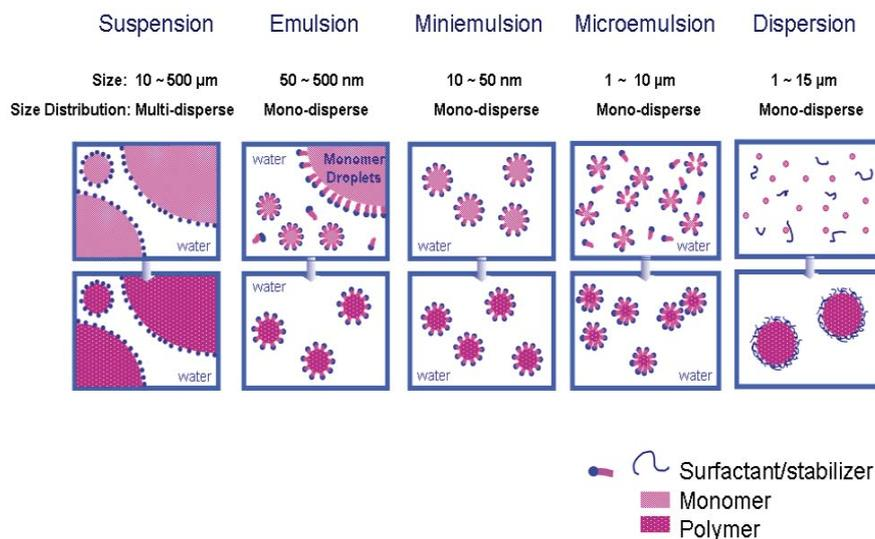
**Scheme 1.** Polymerizations in various aqueous dispersed media.
