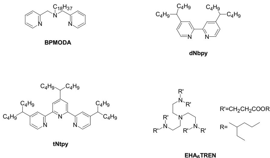
**Scheme 3.** Structures of common ligands used for ATRP in aqueous dispersed media.
