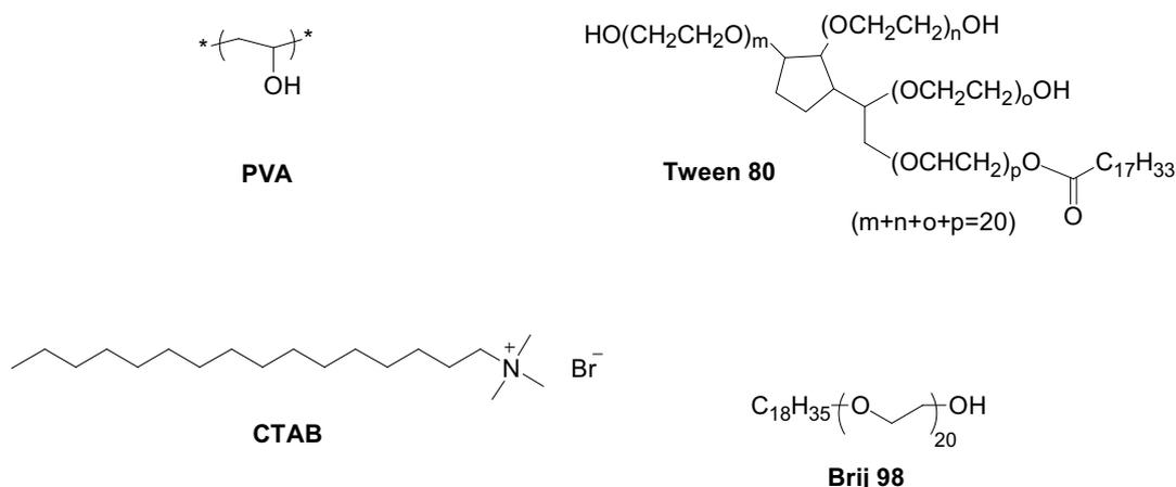
**Scheme 2.** Structures of common surfactants used for ATRP in aqueous dispersed media.
