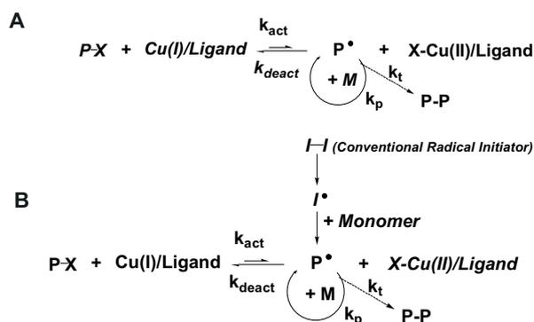
**Scheme 4.** Proposed mechanisms for (A) normal ATRP and (B) reverse ATRP. The activation and deactivation steps proceed with the rate constants  $k_{\text{act}}$  and  $k_{\text{deact}}$ . Generated free radicals propagate and terminate with rate constants  $k_p$  and  $k_t$ . All ingredients present in the initial system are highlighted in italics.
