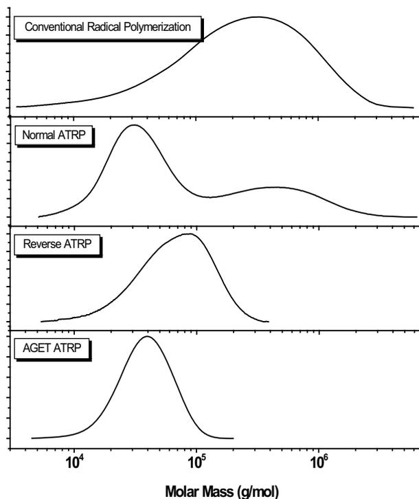
**Figure 2.** Typical GPC traces of the polymers from conventional radical polymerization, normal ATRP, reverse ATRP, AGET ATRP of MMA in microemulsion [76]. Reproduced with permission from the American Chemical Society.
