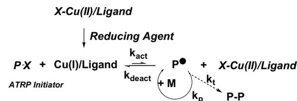
**Scheme 6.** Proposed mechanism for AGET ATRP initiation. All ingredients present in the initial system are highlighted in italics.
