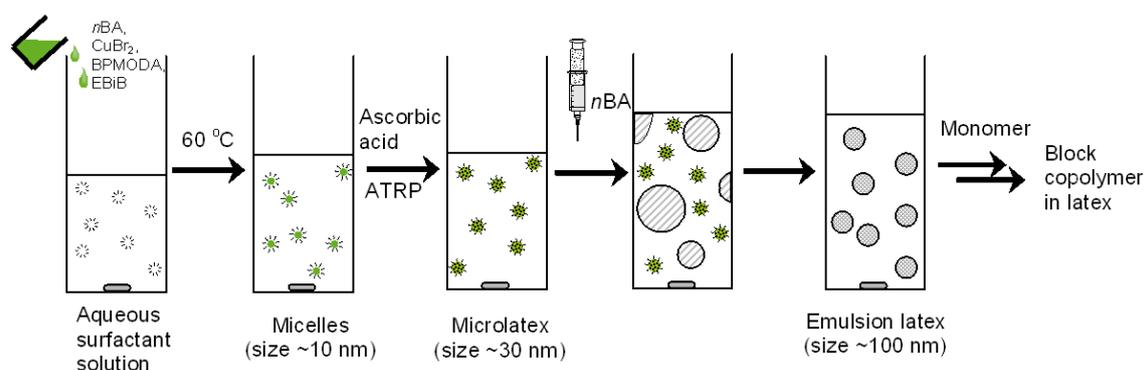
**Scheme 7.** Schematic illustration of ATRP in an emulsion by using the two-step procedure.
