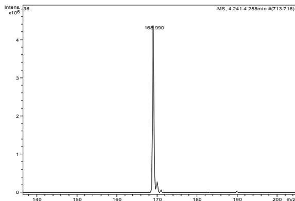
**Figure 2.** Fully automated chip (-) nanoESI HCT MS of standard gallic acid. Solvent: MeOH; ESI/MS parameters: ChipESI: -1.4 kV; capillary exit: -50 V. Back nitrogen pressure 0.30 p.s.i. Nitrogen nebulizer on MS at 50 p.s.i.
