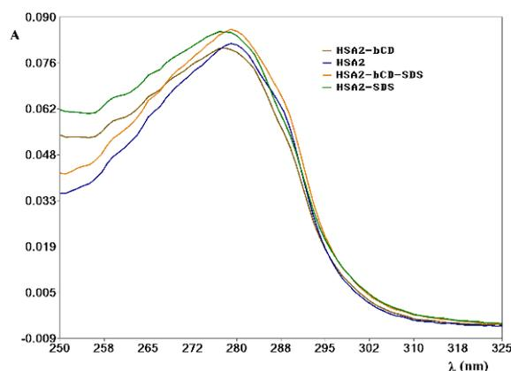
**Figure 4.** UV spectra of HSA2 in the presence of  $\beta$ -CD and/or SDS. UV spectra of HSA1 (native conformer), in the presence of  $\beta$ -CD and/or SDS
