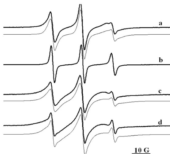
**Figure 6.** EPR spectra of CAT16 in solutions of (a) HSA1, (b) HSA1 +  $\beta$ -CD, (c) HSA1 + SDS, (d) HSA1 +  $\beta$ -CD/SDS mixture. Simulated spectra are shown as thin lines below the experimental ones.
