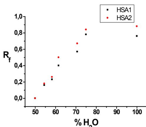
**Figure 3.**  $R_f$  values for albumin samples HSA1 and HSA2 corresponding to chromatographic systems silica gel impregnated with paraffin oil; eluent: water/acetone/2-propanol.
