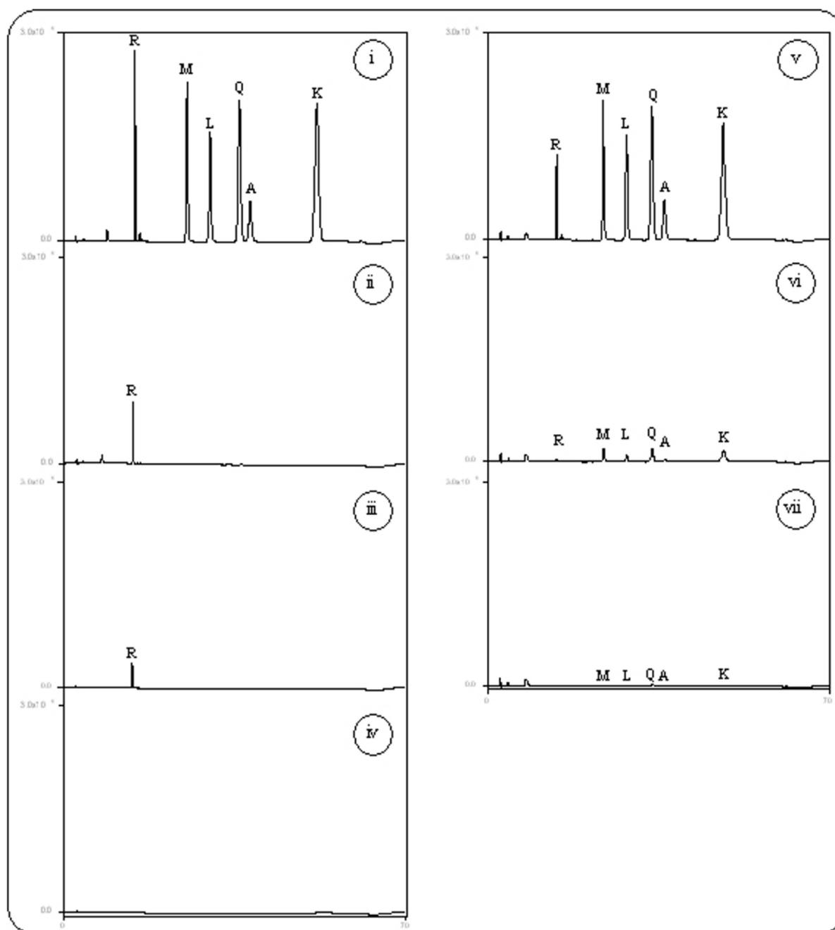
**Figure 4.** HPLC-PDA chromatograms of samples collected from the SPE of flavonoid standard mixture applied at  $\lambda_{\max}$  370 nm using 4-VP-co-EDMA as SPE sorbent: (i) flavonoid standard mixture, (ii) flow through, (iii) washing 1, (iv) washing 2, (v) elution 1, (vi) elution 2, (vii) elution 3. R = rutin, M = myricetin, L = luteolin, Q = quercetin, A = apigenin, K = kaempferol
