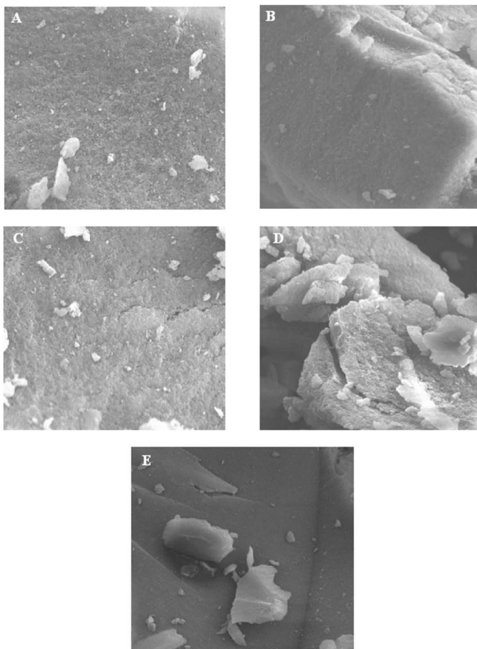
**Figure 3.** Scanning Electron Microscope Micrographs of polymeric SPE materials: (A) 4-VP-co-EDMA, (B) methacrylic acid-co-EDMA, (C) acrylamide-co-EDMA (6 + 30), (D) acrylamide-co-EDMA (4 + 40), (E) acrylamide-co-DVB. Magnification of each micrograph is 10  $\mu\text{m}$ .
