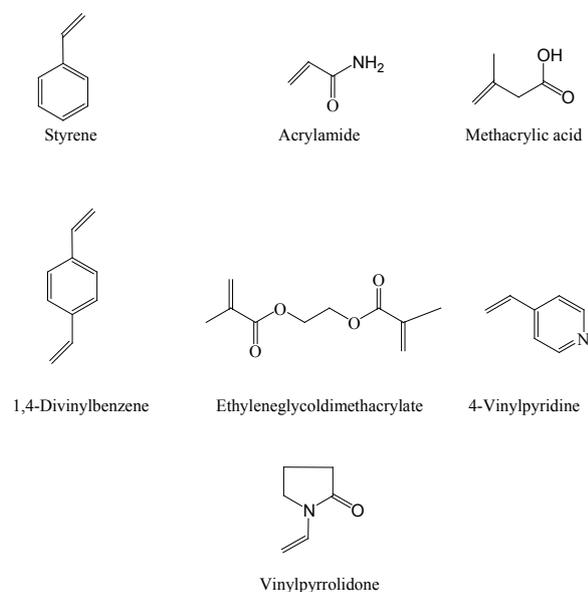
**Figure 1.** Molecular structures of some monomers and cross-linkers
