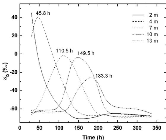
**Figure 3.** Deuterated water flow movement in the constructed wetland bed.
