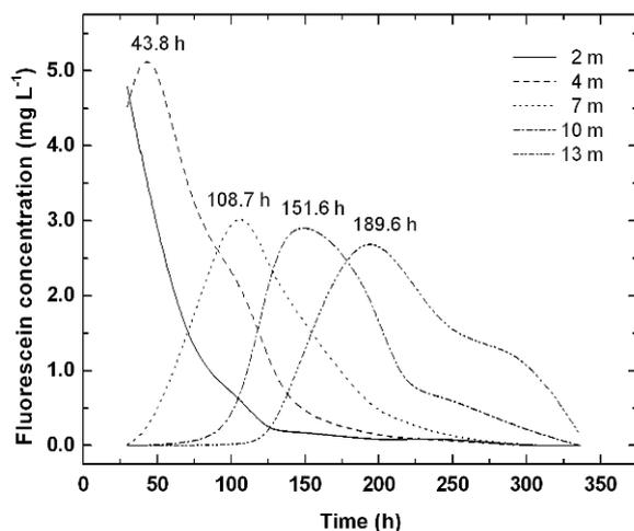
**Figure 2.** Fluorescein flow movement in the constructed wetland bed.
