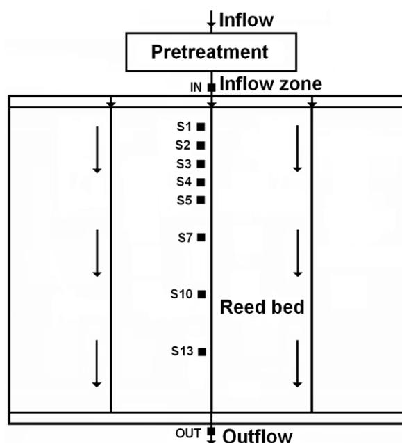
**Figure 1.** Scheme of the constructed wetland reed bed with the pretreatment section.
