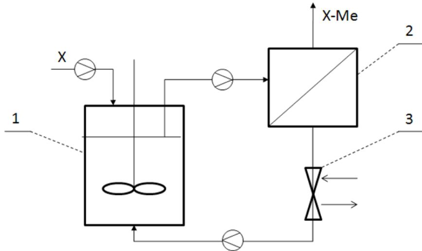
**Figure 1.** Flowchart of the production of mineral feeds additives based on algal biomass. (1): Reactor/biosorber (here the biosorption process takes place), (2): Filter (here the separation of the biomass from permeate takes place), (3): Valve [13].
