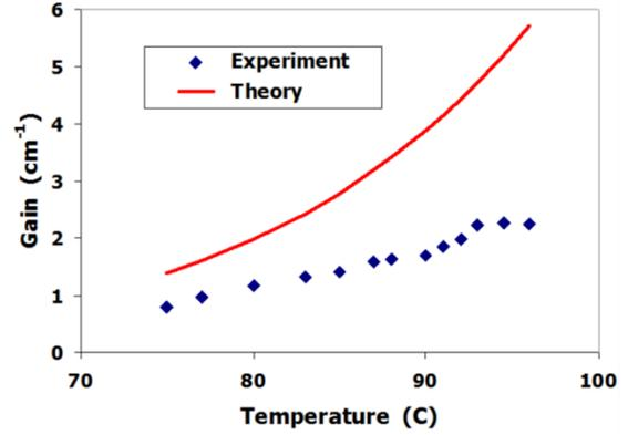
Figure 13. Cs amplifier experimental gain coefficient vs vapor temperature – comparison with theory.
