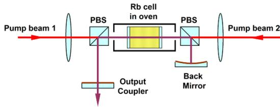
**Figure 6.** Schematic of the experimental setup. The polarizing beam splitters (PBS) are used so that the polarization of the laser is orthogonal to the polarization of two pump beams.
