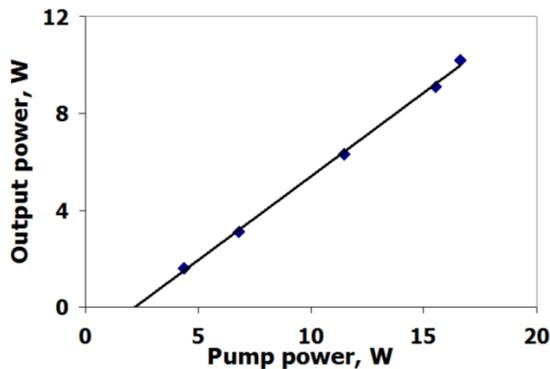
**Figure 4.** Output power of the Cs laser as a function of input pump power. The data shows 68% optical to optical slope efficiency, a 62% overall efficiency and an output power of 10 watts.
