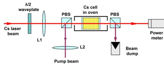
**Figure 12.** Cs amplifier - experimental apparatus.
