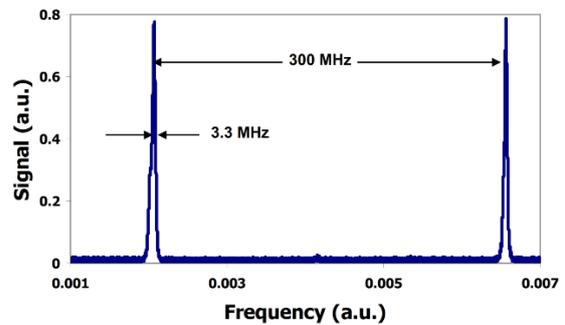
**Figure 16.** High resolution spectrum of the Cs laser output obtained with a Coherent interferometer (FSR 300 MHz) showing a single mode operation with a linewidth less than 3.3 MHz.
