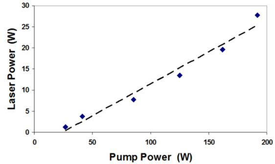
**Figure 11.** Cs laser output power dependence on pump power at an optimal temperature of 120°C.
