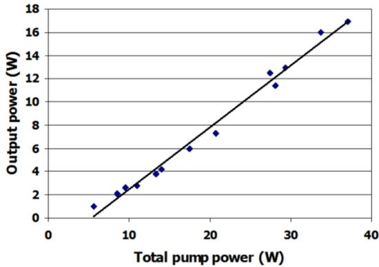
**Figure 7.** Output power of the Rb laser as a function of input pump power.
