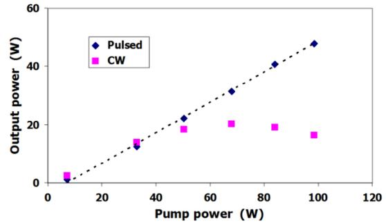
**Figure 9.** Cs laser output power for pulsed (diamonds) and CW (squares) operation depending on the pump power. The dashed line is a linear fit to the pulsed operation data showing a 52% slope efficiency.
