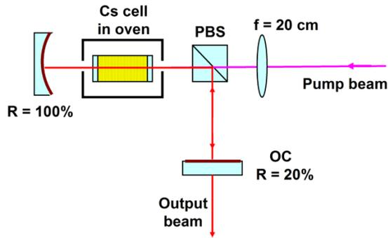
**Figure 3.** Schematic diagram of the diode pumped cesium laser.
