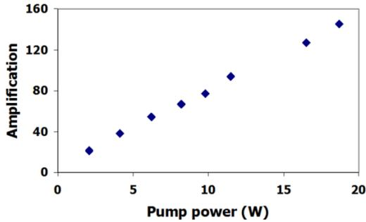
**Figure 14.** Cs amplifier small signal amplification factor vs pump power. Input signal is 10 mW,  $T = 94^\circ\text{C}$ .
