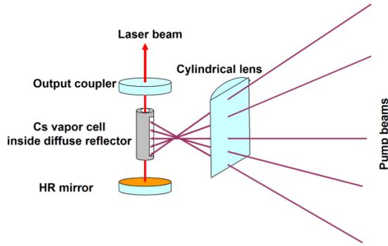
**Figure 10.** Schematic diagram of the transverse pumped Cs laser configuration.
