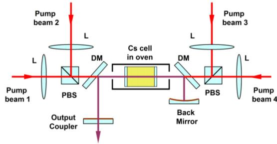
**Figure 8.** Schematic diagram of the Cs laser configuration. DM are dichroic mirrors, PBS are polarizing beam combiners and L are lenses.
