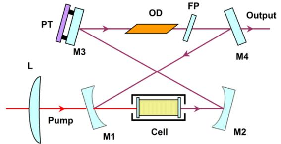
**Figure 15.** Ring cavity Cs laser setup: M1, M2, M3 and M4 – cavity mirrors, OD – optical diode, FP – Fabry-Perot etalon, PT – piezo transducer, Cell – Cs vapor cell in oven, L – focusing lens.
