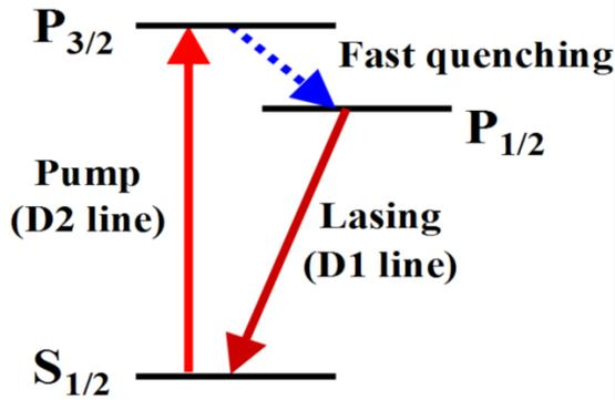
**Figure 2.** Alkali Lasers Energy Level Diagram.
