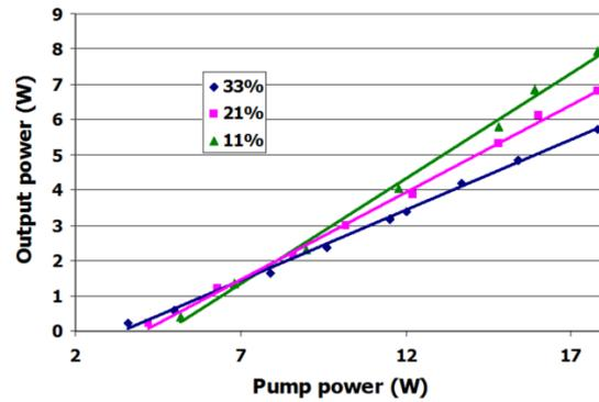
**Figure 5.** Output power of the Rb laser as a function of input pump power for different output couplers (33%, 21% and 11%). For the optimal output coupler of 11% the data shows 60% optical to optical slope efficiency, a 45% overall efficiency and an output power of 8 watts.
