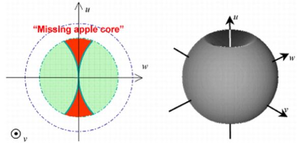
**Figure 3.** Representation of the optical transfer function of a tomographic diffractive microscope with specimen rotation. The frequency support is almost spherical, but exhibits a set (in red) of uncaptured frequencies, which as the shape of an apple core.
