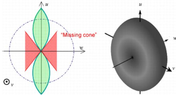
**Figure 2.** Representation of the optical transfer function of a tomographic diffractive microscope with illumination rotation. While the resolution is doubled with respect to a conventional transmission microscope, the frequency support exhibits a missing-cone (in red) of uncaptured frequencies, responsible for the poorer resolution along the optical axis.
