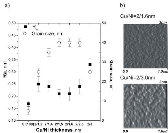
**Figure 3.** Surface roughness and grain size determined from the area of  $1 \mu\text{m}$  as a function of Cu/Ni multilayer period thickness; b) a two-dimensional image of surface topography for multilayers with the lowest roughness (top/bottom?) and the highest roughness, respectively.
