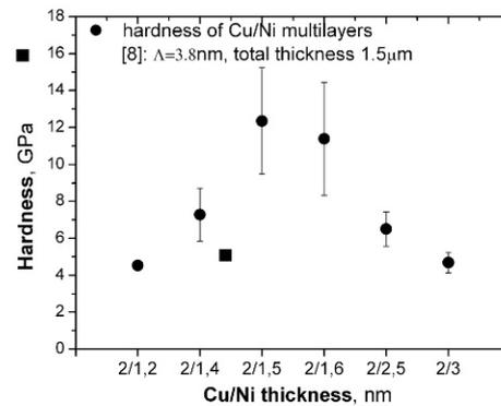
**Figure 5.** Nano-hardness of the multilayer as a function of Cu/Ni period thickness.
