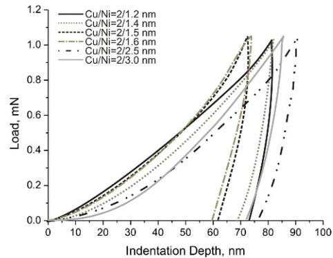
**Figure 4.** Sample loading and unloading curves for Cu/Ni multilayers
