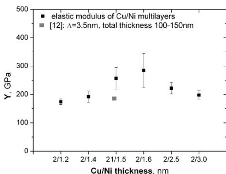
**Figure 6.** Young's modulus for the multilayer as a function of Cu/Ni period thickness.
