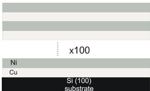
**Figure 1.** Schematic of the arrangement of sublayers in the multilayers examined.
