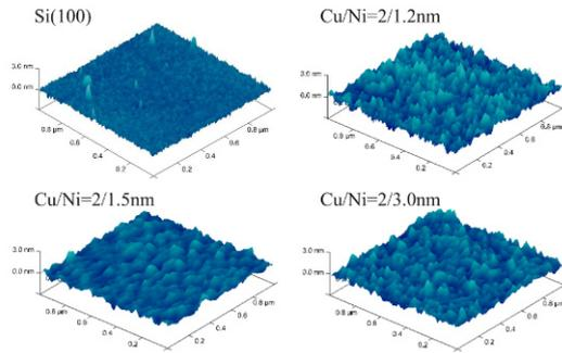
**Figure 2.** Three-dimensional images of the surface topography of substrate and sample Cu/Ni multilayers subjected to AFM examinations.
