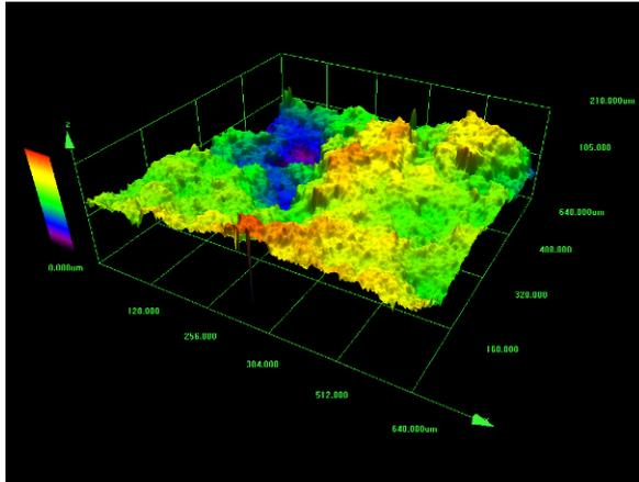
**Figure 1.** Confocal reconstruction of the surface relief of the fracture sample made of hydrated cement paste.
