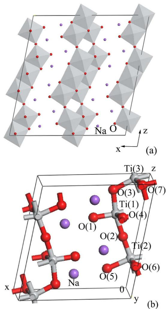
**Figure 1.** Crystal structures of  $\text{Na}_2\text{Ti}_3\text{O}_7$  (a) Layered polyhedron structure on  $xz$  plane; (b) Unit cell. Red, gray and purple spheres indicate O, Ti and Na atoms, respectively. To make a clear description, Ti (1–3) and O (1–7) represent corresponding Ti and O atoms, respectively.
