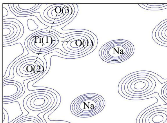
**Figure 4.** The electron density map on the (0, 4, 0) plane of  $\text{Na}_2\text{Ti}_3\text{O}_7$ . Contour lines are drawn at 3 electrons/ $\text{\AA}^3$  intervals.
