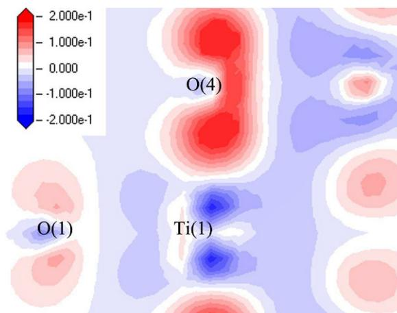
**Figure 5.** The electron density difference map of  $\text{Na}_2\text{Ti}_3\text{O}_7$ . The map is vertical to the [1 0 0] direction. The scale of this map (32 contour lines) is from -0.2 to 0.2 electrons/ $\text{\AA}^3$ . Red or blue areas denote negative or positive electron density relative to the atom electron density respectively.
