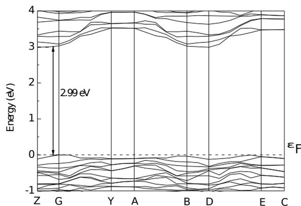
**Figure 2.** Calculated band structure of  $\text{Na}_2\text{Ti}_3\text{O}_7$ . The Fermi energy  $\epsilon_F$  is taken as the zero of energy marked with dash lines.
