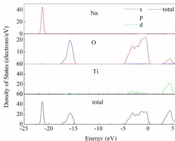
**Figure 3.** TDOS and PDOS of  $\text{Na}_2\text{Ti}_3\text{O}_7$  in which s, p, d partial and total density of state of different atoms and unit cell are drawn in blue, red, green and black lines, respectively. The Fermi level is set as 0 eV.
