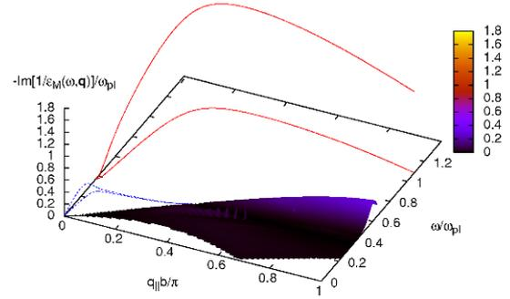
**Figure 5.** Energy-loss functions  $-\Im m[1/\epsilon_M(\mathbf{q}, \omega)]/\omega_{pl}$  for  $q_{\perp} = 0.2\pi/a$ . Lines indicate the strength  $Z(\mathbf{q})\pi/\omega_{pl}$  of  $\delta$ -peaks in the energy-loss function that belong to collective mode dispersions  $\Omega_1(\mathbf{q})$  (dashed line) and  $\Omega_2(\mathbf{q})$  (solid line).
