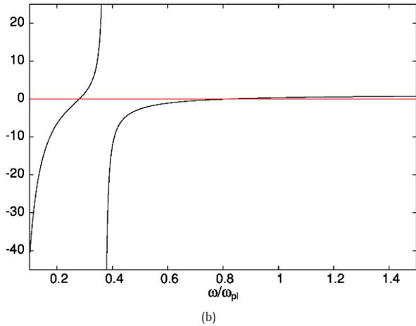
**Figure 4.** Frequency dependence of  $\Re\epsilon_M(\mathbf{q}, \omega)$  (solid line) and  $\Im\epsilon_M(\mathbf{q}, \omega)/10$  (dashed line) for macroscopic dielectric function (15) with  $q_{\perp} = 0.2\pi/a$  and  $q_{\parallel} = 0.05\pi/b$ .
